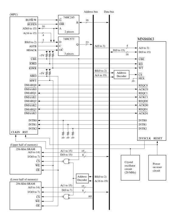
■ Application Circuit Example #2. Sample Connections to Image Bus
