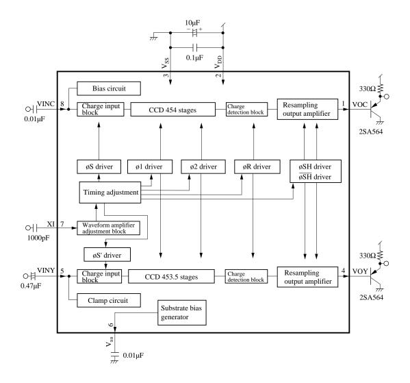
Note: If the external capacitor attached to pin 6 is a electrolytic capacitor, connect the negative pole to pin 6.
