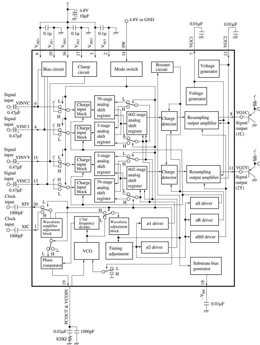
Note: If the capacitor attached to pin 18 has a polarity, attach the negative pole to pin 18.
