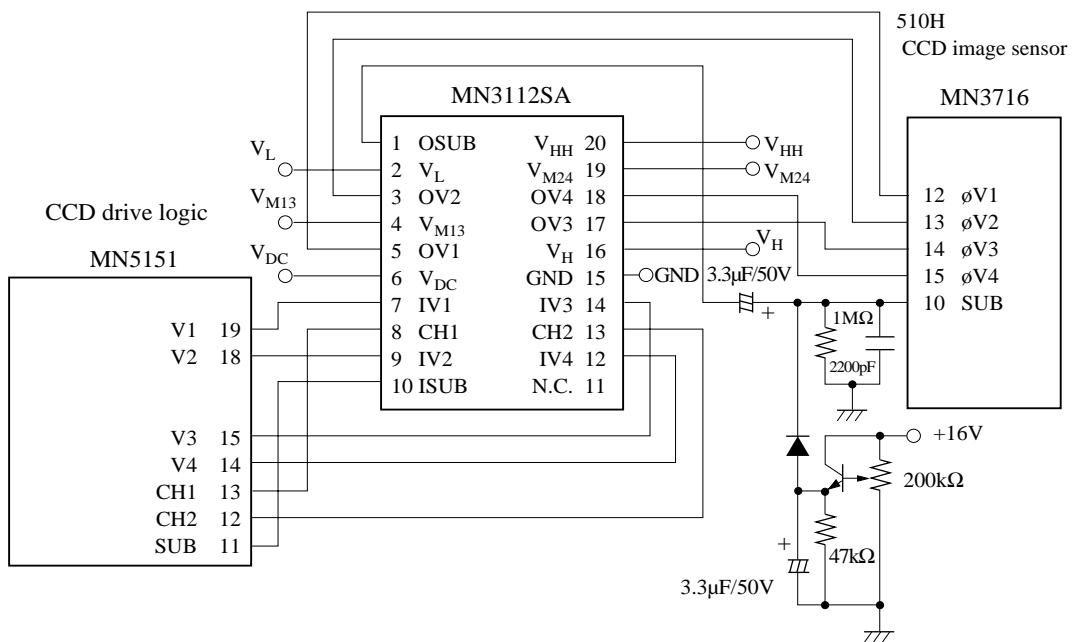
Note \*1: Connect a bypass capacitor as close as possible to each of the MN3112SA's power supply pins (V<sub>HH</sub>, V<sub>H</sub>, V<sub>M13</sub>, V<sub>M24</sub>, V<sub>L</sub>, V<sub>DC</sub>).
