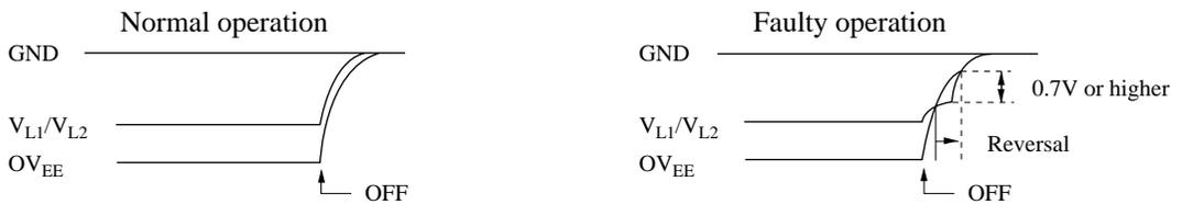
As the above sketch illustrates, allowing  $OV_{EE}$  to exceed  $V_{L1}$  and  $V_{L2}$  by more than 0.7 V produces the risk of applying a forward bias to the PN junction, turning on the parasitic transistor, and generating an overcurrent that produces latch-up.
