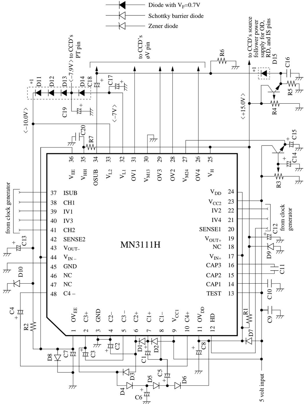
The booster circuit's electrolytic capacitors must have little impedance fluctuation at low temperatures.
