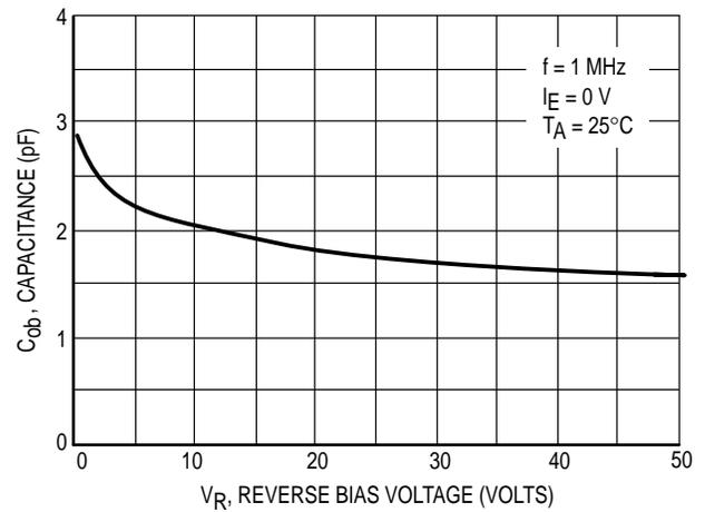
Figure 4. Output Capacitance
