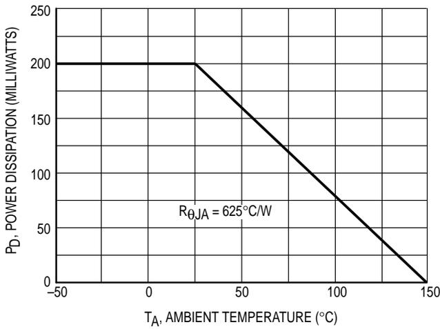
Figure 1. Derating Curve
