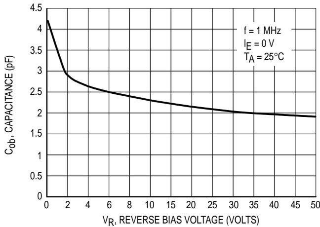
Figure 19. Output Capacitance
