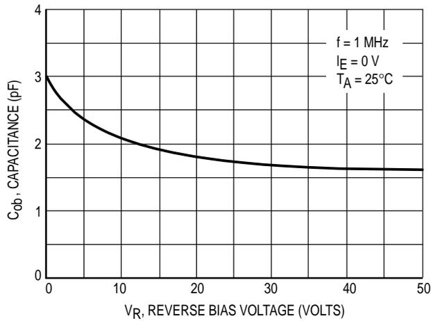
Figure 9. Output Capacitance
