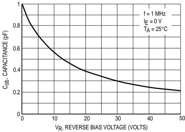
Figure 14. Output Capacitance
