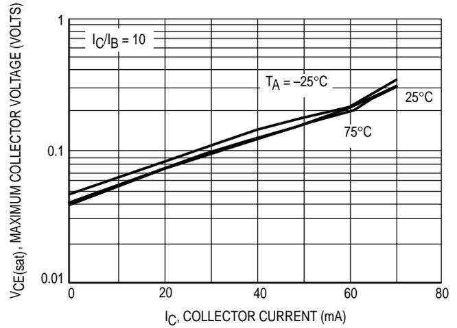
Figure 2. V<sub>CE(sat)</sub> versus I<sub>C</sub>
