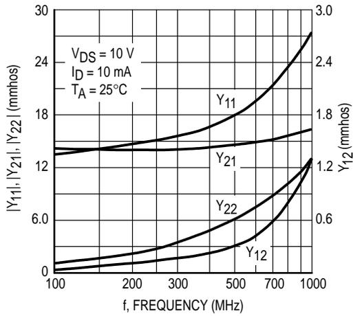
Figure 6. Common-Gate Y Parameter Magnitude versus Frequency
