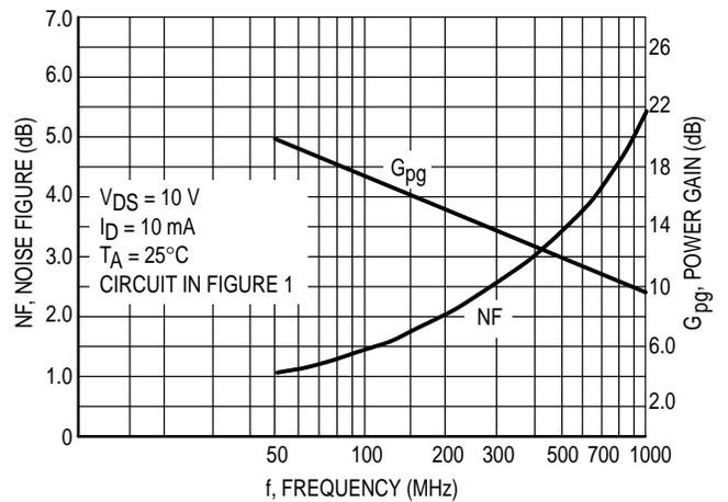
Figure 11. Noise Figure and Power Gain versus Frequency
