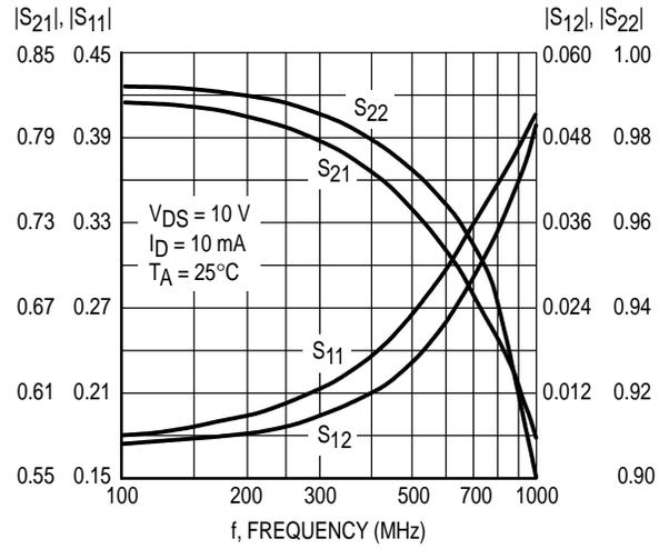
Figure 7. Common-Gate S Parameter Magnitude versus Frequency
