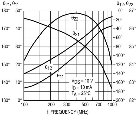
Figure 8. Common-Gate Y Parameter Phase-Angle versus Frequency
