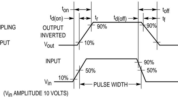
Figure 2. Switching Waveform
