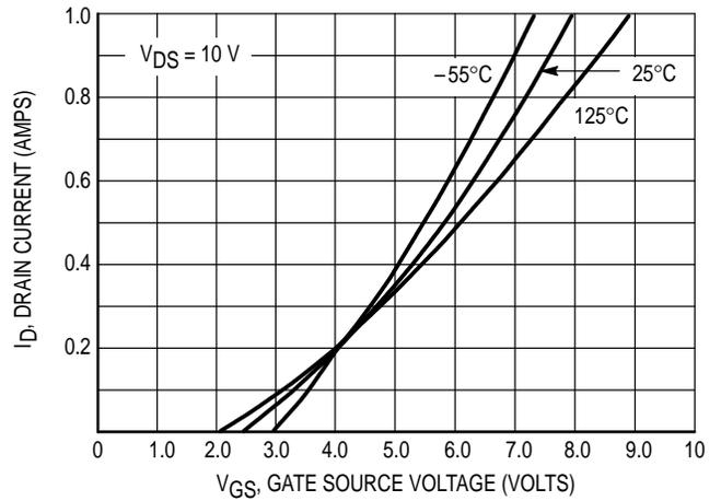
Figure 4. Transfer Characteristics
