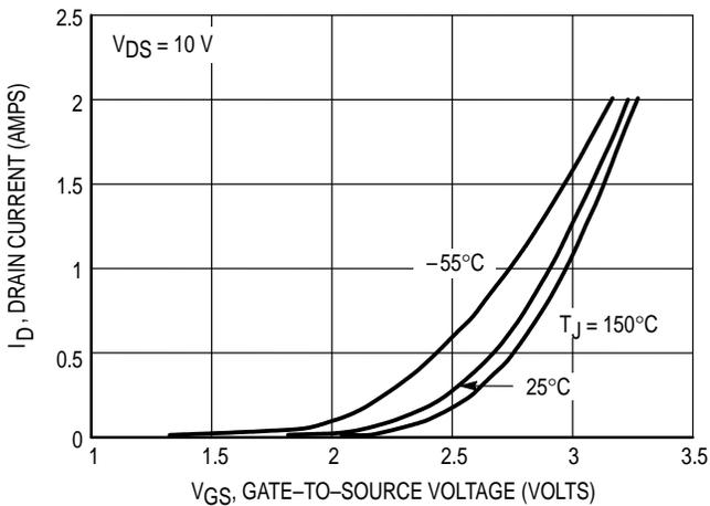
Figure 1. Transfer Characteristics
