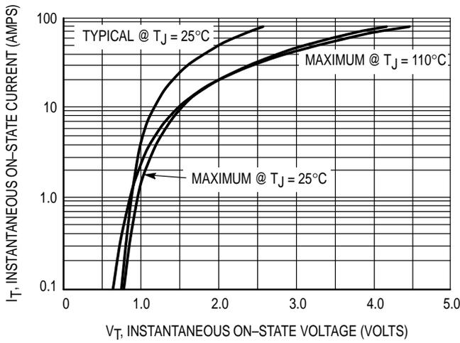
Figure 3. On-State Characteristics
