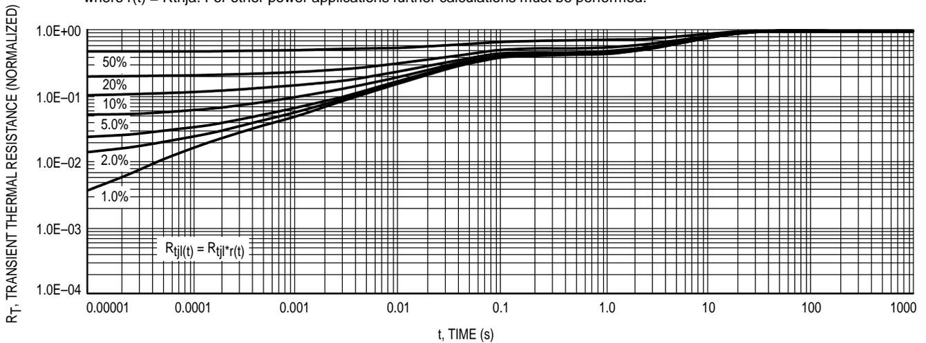
Figure 9. Thermal Response — Junction to Case
