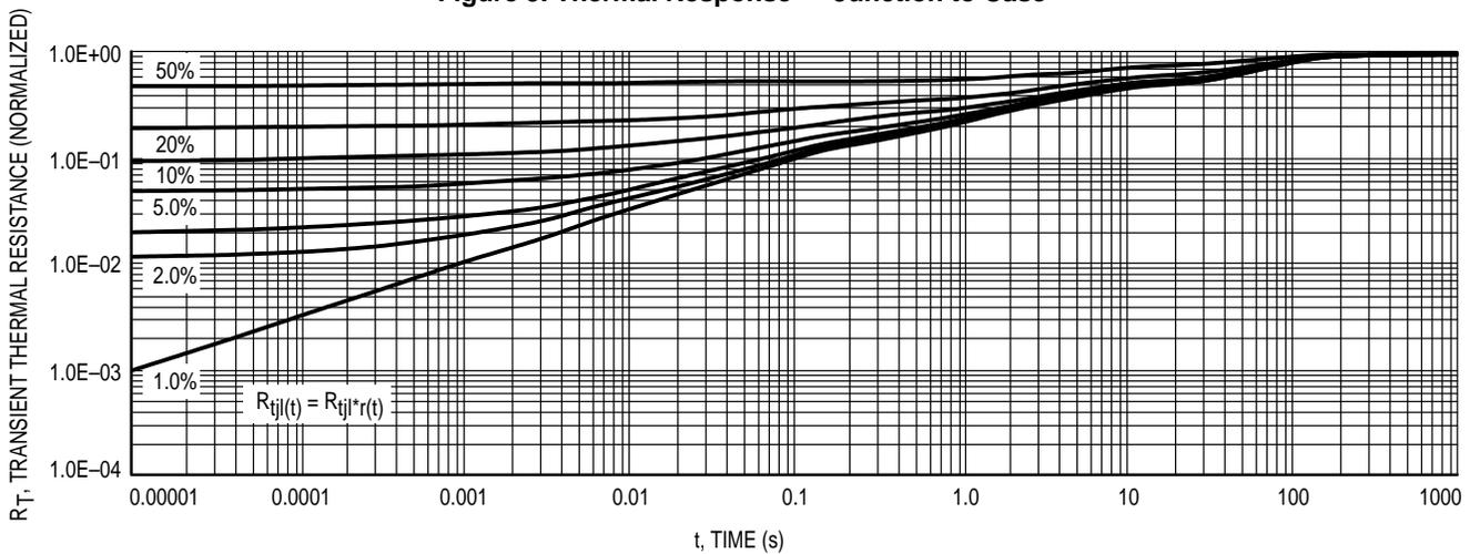
Figure 10. Thermal Response — Junction to Ambient
