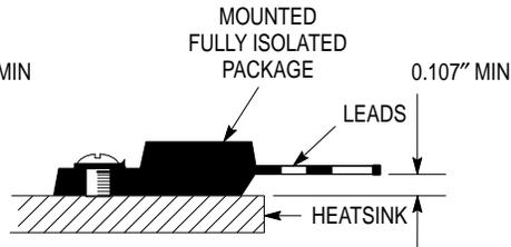
Figure 5. Screw Mounting Position for Isolation Test Number 3
