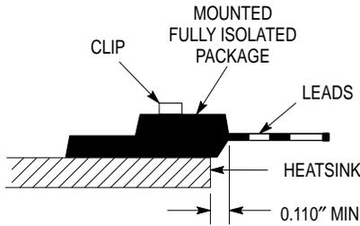
Figure 3. Clip Mounting Position for Isolation Test Number 1
