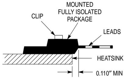
Figure 7. Clip Mounting Position for Isolation Test Number 1
