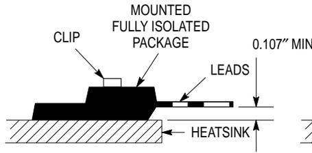
Figure 8. Clip Mounting Position for Isolation Test Number 2
