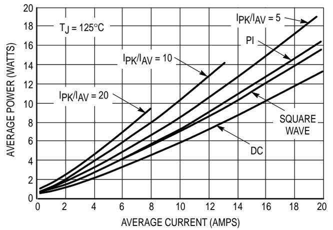
Figure 4. Average Power Dissipation and Average Current
