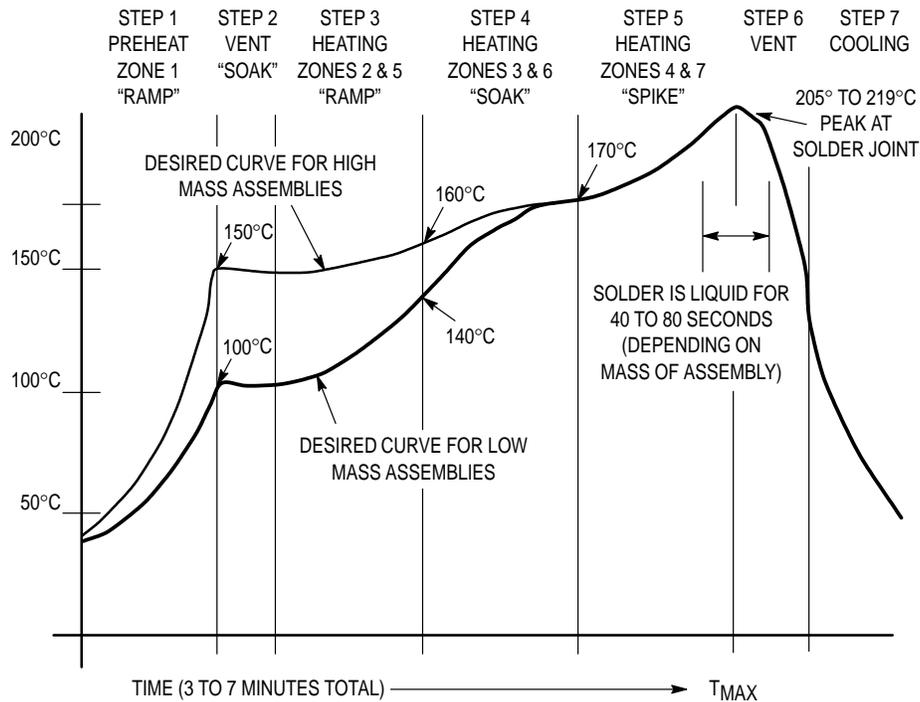
**Figure 5. Typical Solder Heating Profile for D<sup>2</sup>PAK**
