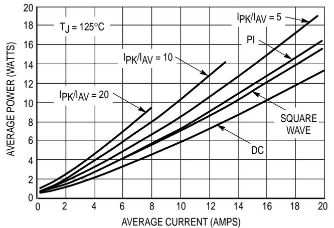
Figure 4. Average Power Dissipation and Average Current
