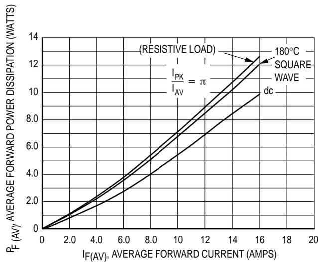
Figure 5. Power Dissipation
