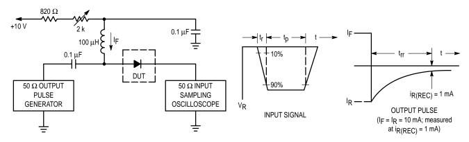
Notes: 1. A 2.0  $k\Omega$  variable resistor adjusted for a Forward Current (I<sub>F</sub>) of 10 mA.
