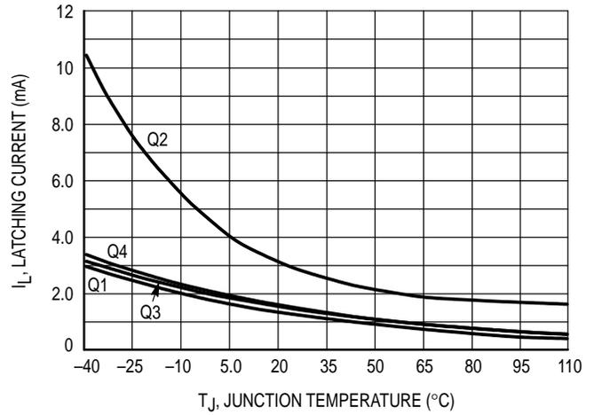
**Figure 8. Typical Latching Current versus Junction Temperature**
