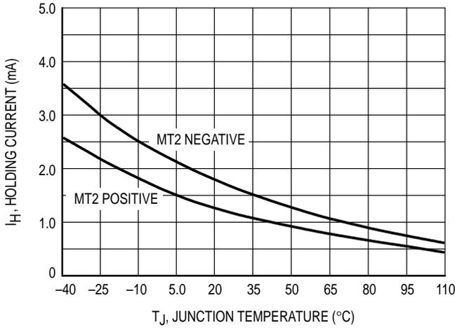
**Figure 7. Typical Holding Current versus Junction Temperature**
