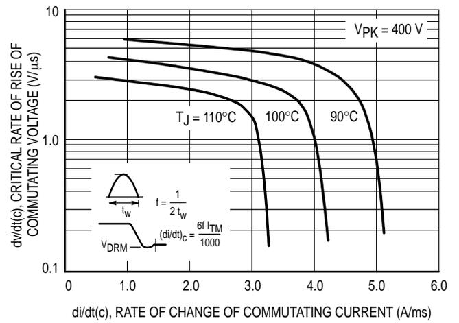
**Figure 10. Critical Rate of Rise of Commutating Voltage**
