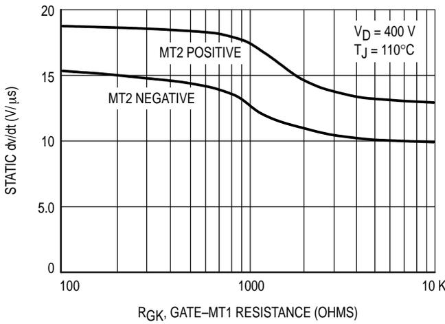
**Figure 9. Exponential Static dv/dt versus Gate-MT1 Resistance, MT2(+)**
