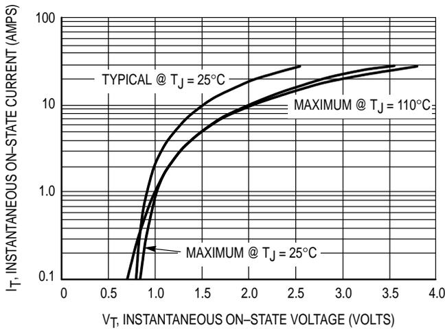
Figure 3. On-State Characteristics
