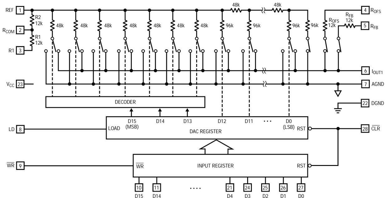
**Figure 1. The LTC1597 16-bit CMOS DAC uses a precision thin-film modified R/2R architecture to provide unsurpassed accuracy and stability. Accurate 4-quadrant multiplication applications are now possible with on-chip resistors R1, R2 and  $R_{OFS}$ . A built-in deglitcher reduces glitch impulse to 1nV-s.**
