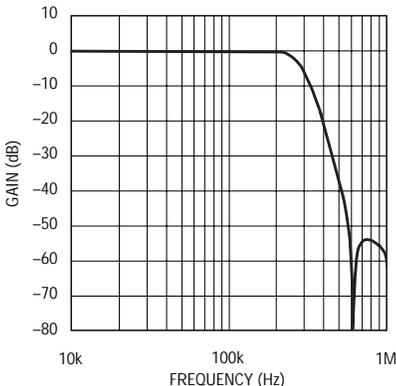
**Figure 6. Gain response of Figure 5's circuit**
