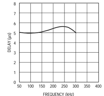
**Figure 8. Group delay response of Figure 5's circuit**
