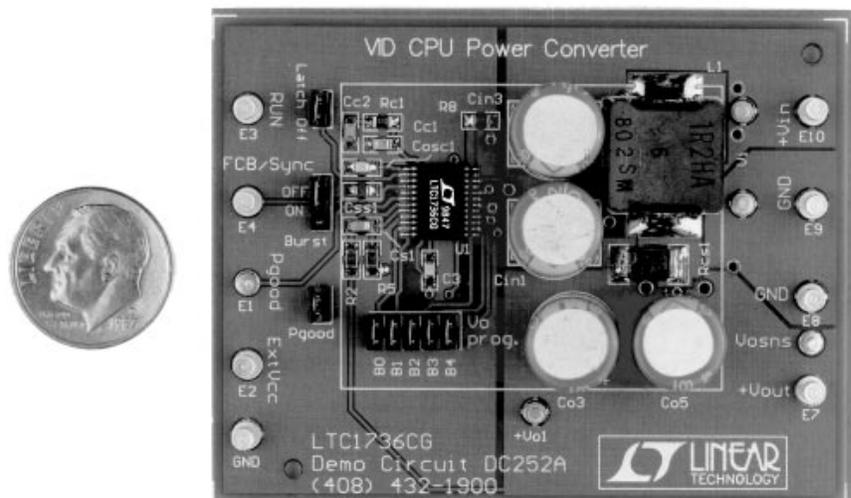
**Figure 1. LTC1736 evaluation circuit: a complete 5V–24V to 0.9V–2V/12A converter in 2.15in<sup>2</sup> of PC board space**
