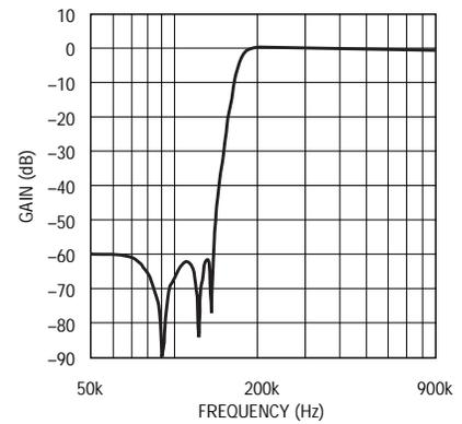
**Figure 10. Frequency response of Figure 9’s circuit**
