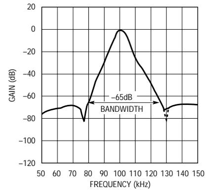
Figure 6. Measured amplitude response of Figure 5's filter
