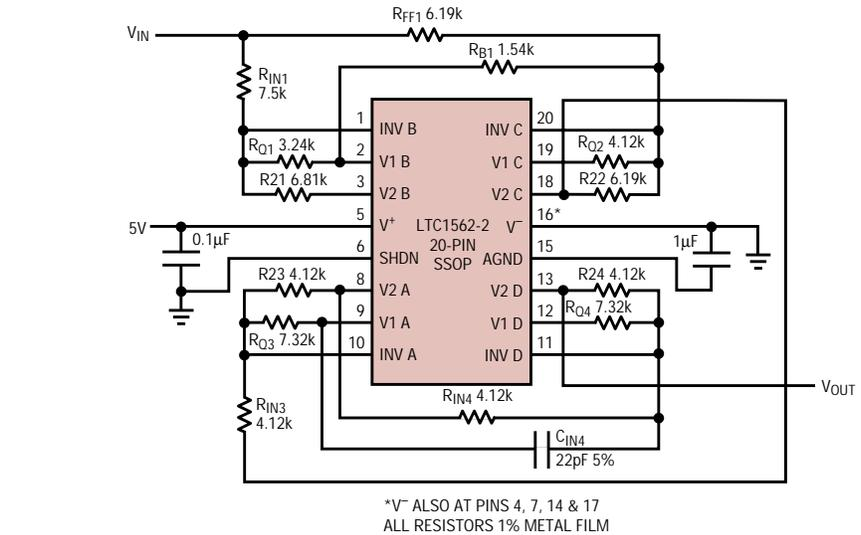
**Figure 5. 256kHz linear-phase 6th order lowpass filter**
