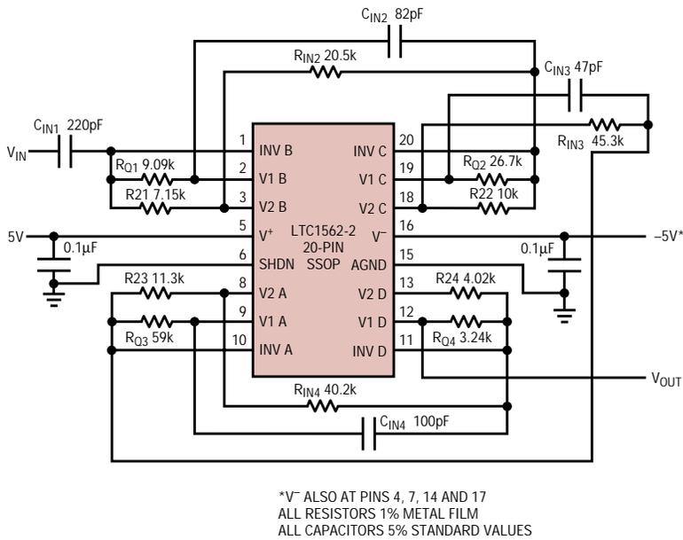
**Figure 9. 175kHz 8th order elliptic highpass filter**
