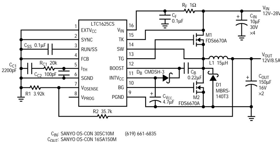
Figure 1. 100W, 12V, 8.5A supply
