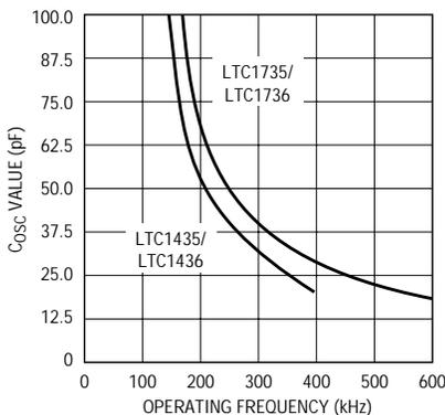
Figure 2. C<sub>osc</sub> value vs frequency for the LTC1435/36 and the LTC1735/36
