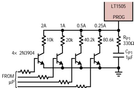
Figure 3. Programming of battery-charge current
