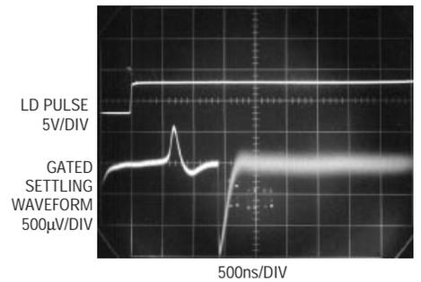
**Figure 4. When used with the LT1468 and a 20pF feedback capacitor (see Figure 3), the LTC1597 can settle in an amazing 1.7 $\mu\text{s}$  to within 0.0015%. The top trace shows the LD pulse; the bottom trace shows the gated settling waveform settling to 1LSB in 1.7 $\mu\text{s}$ .**
