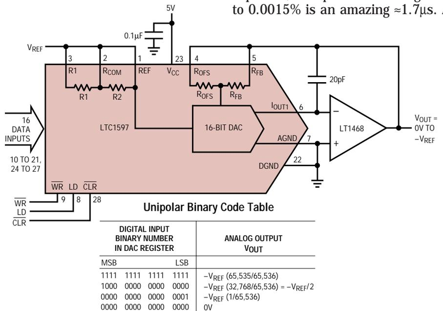
**Figure 3. With a single external op amp, the LTC1597 performs 2-quadrant multiplication with  $\pm 10\text{V}$  input and 0V to  $-V_{REF}$  output. With a fixed  $-10\text{V}$  reference, it provides a precision 0V to 10V unipolar output.**
