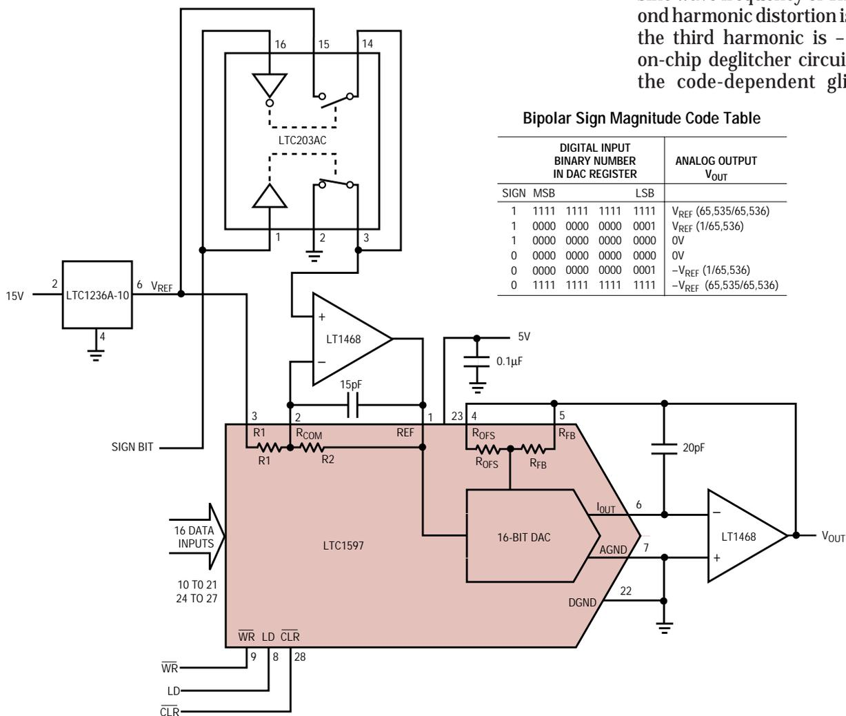
Figure 8. This 17-bit sign-magnitude DAC uses the LTC1597 in its unipolar mode with the reference bit inverted ( $-V_{REF}$ ) for the output range 0V to  $V_{REF}$ . When the sign bit changes, the analog switch changes the reference input polarity to noninverting ( $V_{REF}$ ) for the output range 0V to  $-V_{REF}$ . The resulting circuit produces an impressive bipolar zero error of 140µV (0.92LSB) max at room temperature—less than 1LSB at 17 bits.
