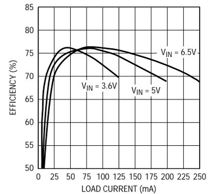
**Figure 7.** Efficiency of Figure 6's SEPIC reaches 77%.
