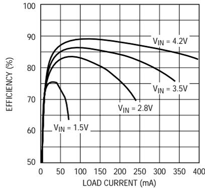
Figure 2. Efficiency of Figure 1's boost converter
