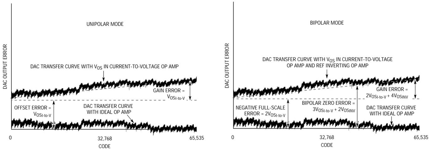
**Figure 10.** The effect of op amp offset on the LTC1597 gain and offset errors in unipolar mode (left) and bipolar mode (right); op amp offset has virtually no effect on DAC linearity; it merely shifts the end points.
