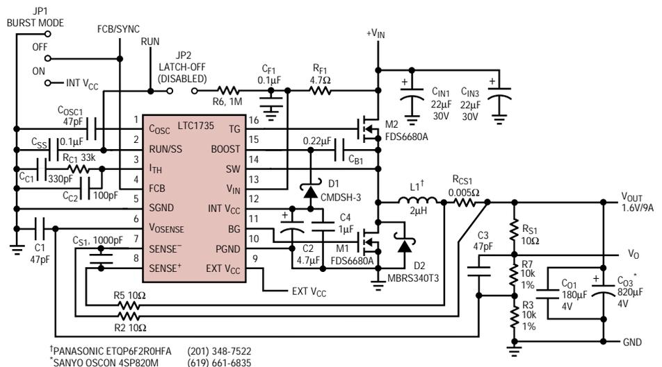
**Figure 5. High efficiency 1.6V/9A CPU power supply**
