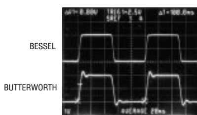
Figure 4. Oscilloscope of square wave response; top trace is the LTC1065 Bessel filter, bottom trace is the LTC1063 Butterworth filter
