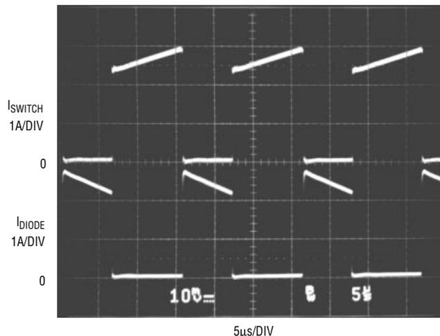
**Figure 24. Positive-to-Negative Converter Switch and Diode Current**
