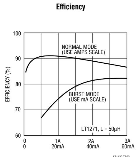
Figure 1. High Efficiency 5V Buck Converter
