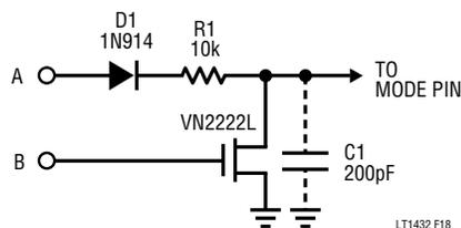
Figure 18. Two Input Mode Drive
