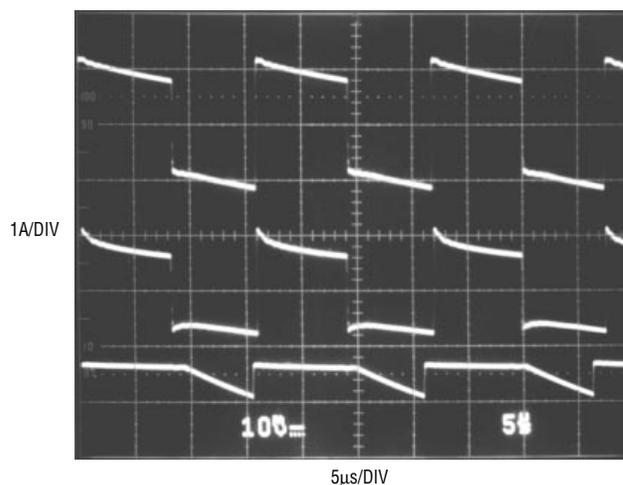
Figure 6. Input Capacitor Current
