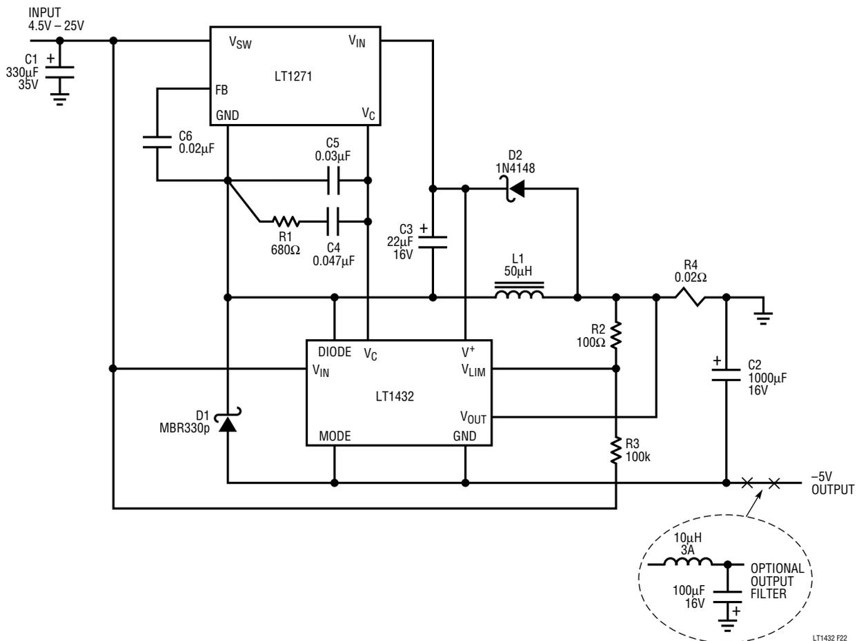
Figure 22. Positive-to-Negative Converter
