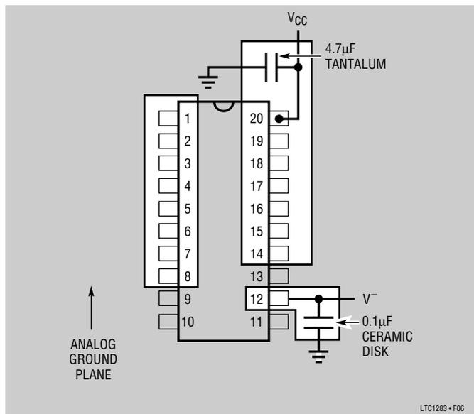
Figure 6. Example Ground Plane for the LTC1283
