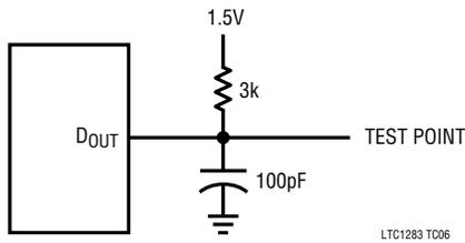
Voltage Waveform for  $D_{OUT}$  Rise and Fall Times,  $t_r$  and  $t_f$
