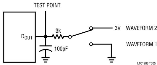
Voltage Waveforms for  $t_{en}$  and  $t_{dis}$
