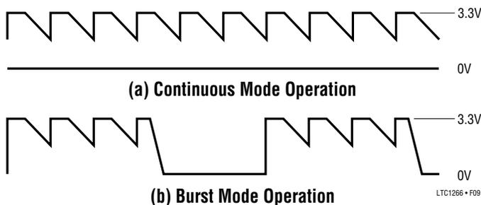
Figure 9.  $C_T$  Waveforms
