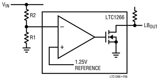
Figure 6. Low-Battery Comparator
