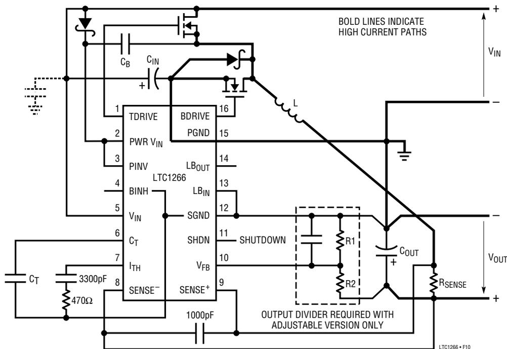
Figure 10. LTC1266 Layout Diagram (See Layout Checklist)
