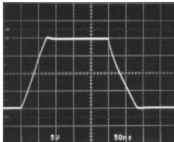
$R_F = R_G = 1k$   $V_{IN} = 20V$  LT1220 • TPC23
