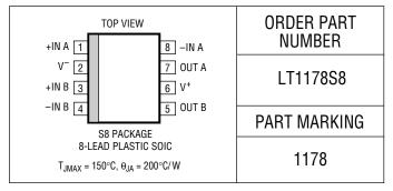
Please note that the LT1178S8 surface mount pinout differs from that of the LT1178 standard plastic or ceramic dual-in-line packages.
