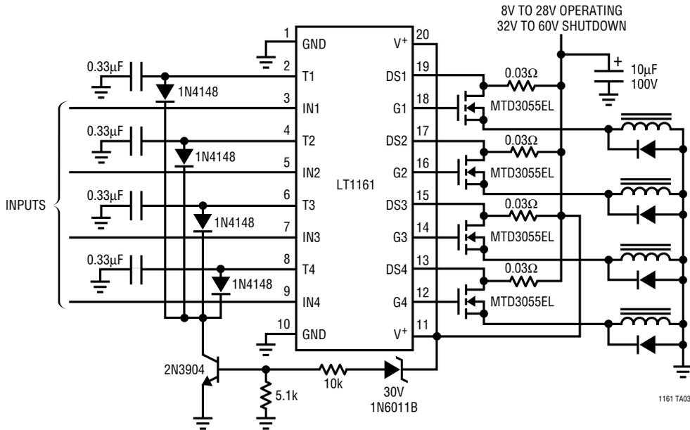
Protected Quad Switch with Mixed Low- and High-Side Driving
