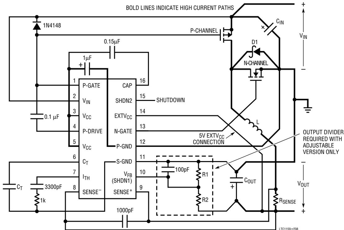
Figure 8. LTC1159 Layout Diagram (N and S Packages)
