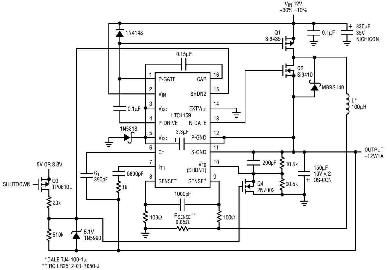
**Figure 15. High Efficiency 12V to -12V 1A Converter**
