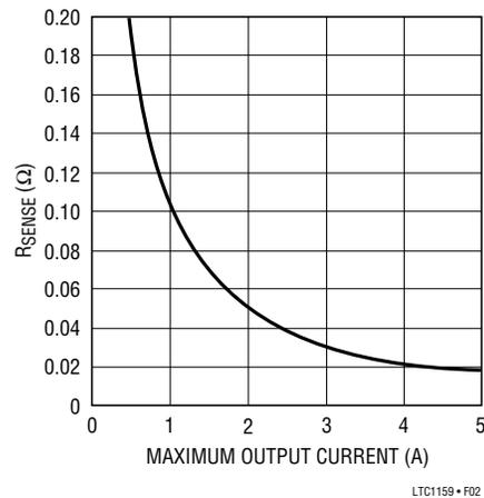
Figure 2. R<sub>SENSE</sub> vs Maximum Output Current
