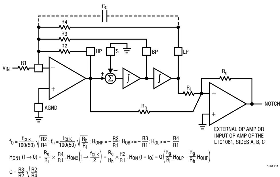
NOTE: FOR  $Q > 5$  AND  $f_{CLK} > 1\text{MHz}$ , ADD  $C_C$  SUCH AS  $C_C \cong \frac{0.16}{R_4 \times 1.2\text{MHz}}$
