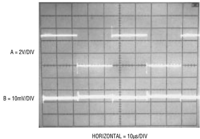
**Figure 2. Typical Clock Feedthrough of the LTC1061 Operating with ±5V Supplies. Top Trace is the Input Clock Swinging 0V to 5V and Bottom Trace is One of the Lowpass Outputs with Zero or DC Input Signals.**
