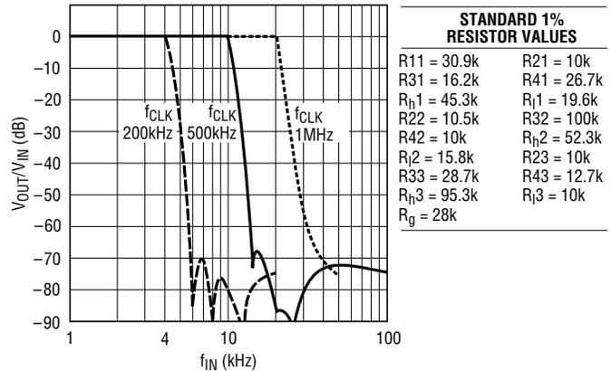
NOTE: ADD A CAPACITOR C ACROSS  $R_g$  TO CREATE A 7TH ORDER LOWPASS SUCH AS  $(1/2\pi R_g C) = (\text{CUTOFF FREQUENCY}) \times 0.38$
