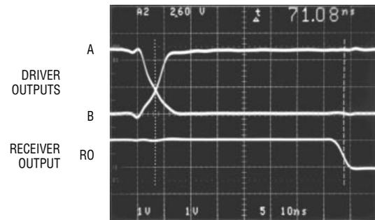
Figure 12. Receiver  $t_{PLH}$
