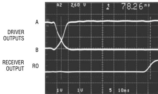
Figure 11. Receiver  $t_{PHL}$
