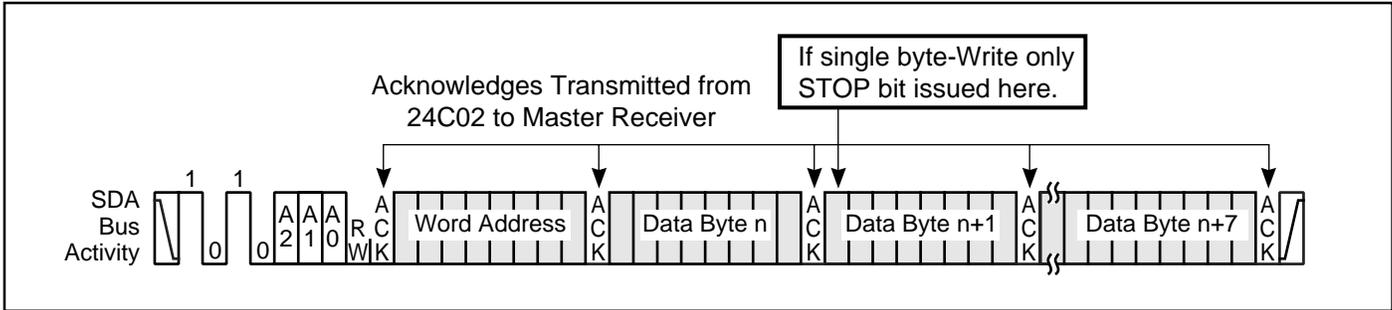
Figure 6. Write Operation
