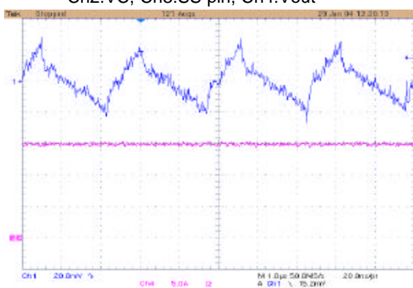
Figure 17 - Output Voltage Ripple @ 15A Ch1:Output, Ch4:lout (5A/Div)
