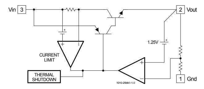
Figure 2 - Simplified block diagram of the IRU1010-25
