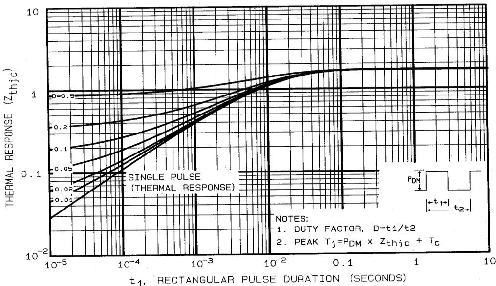
Fig 27. Maximum Effective Transient Thermal Impedance, Junction-to-Case
