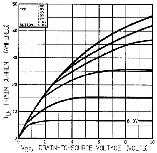
Fig 14. Typical Output Characteristics Post-Irradiation 100K Rads (Si)
