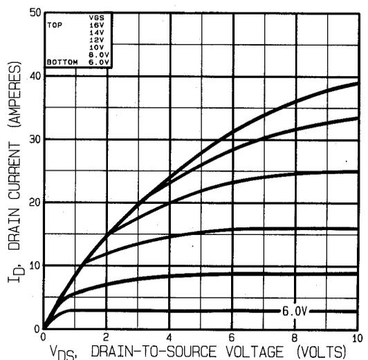
Fig 16. Typical Output Characteristics Post-Irradiation 1 Mega Rads (Si)
