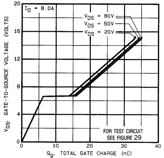
Fig 22. Typical Gate Charge Vs. Gate-to-Source Voltage
