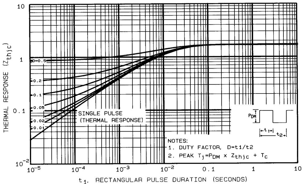
Fig 27. Maximum Effective Transient Thermal Impedance, Junction-to-Case
