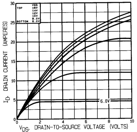
Fig 10. Typical Output Characteristics Post-Irradiation 100K Rads (Si)
