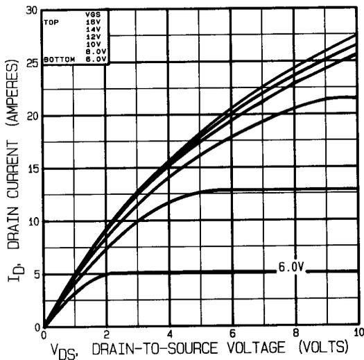
Fig 11. Typical Output Characteristics Post-Irradiation 300K Rads (Si)
