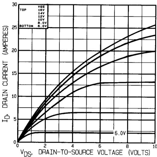
**Fig 15.** Typical Output Characteristics Post-Irradiation 300K Rads (Si)
