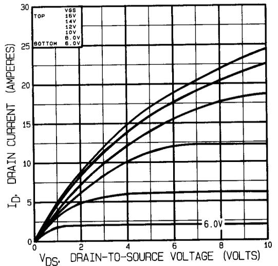
Fig 12. Typical Output Characteristics Post-Irradiation 1 Mega Rads (Si)
