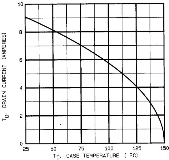
Fig 25. Maximum Drain Current Vs. Case Temperature
