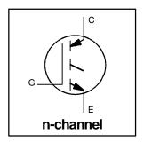
$V_{CES} = 1200V$   $V_{CE(sat)} \le 2.0V$   $@V_{GE} = 15V, I_C = 33A$
