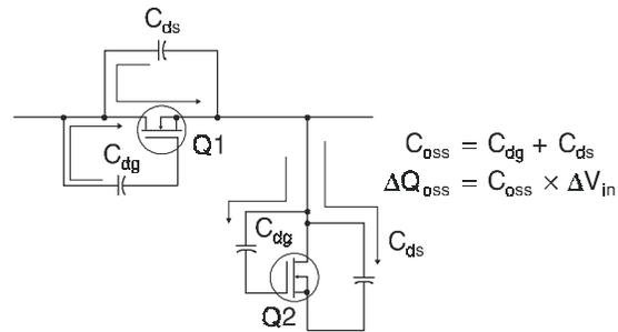
Figure 2:  $Q_{oss}$  Characteristic
