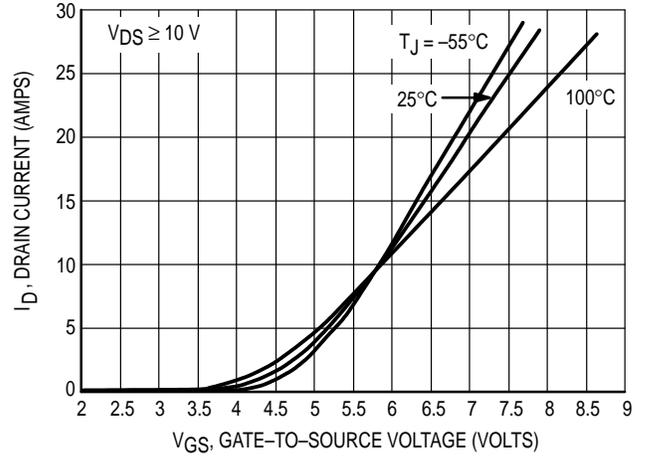
Figure 2. Transfer Characteristics
