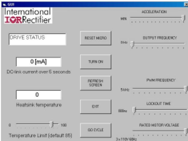
Below said field, at the bottom left, observe the slider with the caption “Temperature limit (default 85)”. Using this slider you may adjust the temperature threshold for the thermal protection. A default value is 85 degrees Centigrade, but you may change this value<sup>1</sup>. Figure 5 shows GUI control screen.
