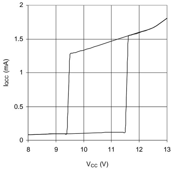
Graph 7.  $I_{QCC}$  vs  $V_{CC}$  (IR2156)
