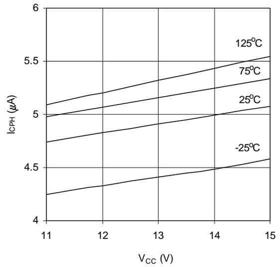
Graph 22.  $I_{CPH}$  vs  $V_{CC}$  vs Temperature (IR2156)
