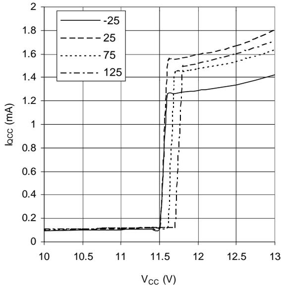
Graph 17.  $I_{QCC}$  vs  $V_{CC}$  vs Temperature (IR2156)
