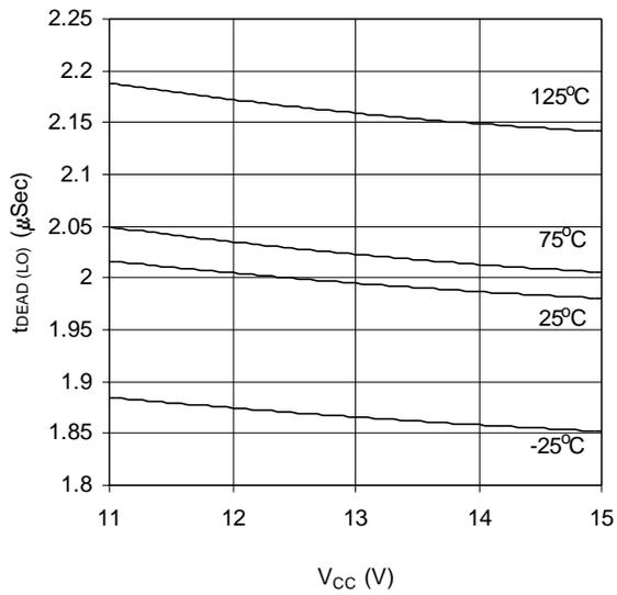
Graph 23.  $t_{DEAD(LO)}$  vs  $V_{CC}$  vs Temperature (IR2156)
