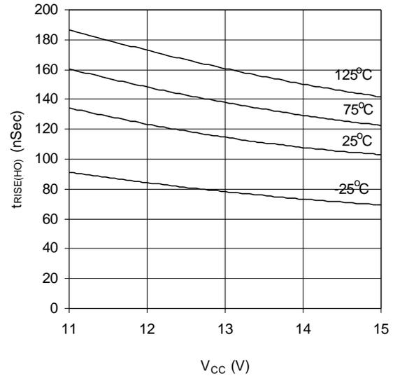
Graph 23.  $t_{RISE(HO)}$  vs  $V_{CC}$  vs Temperature (IR2156)
