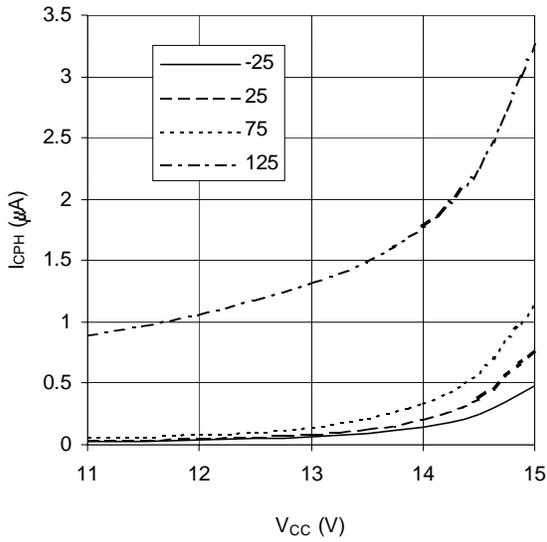
Graph 21.  $I_{CPH}$  vs  $V_{CC}$  vs Temperature (IR2156)
