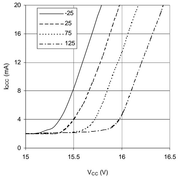
Graph 15.  $I_{QCC}$  vs  $V_{CC}$  vs Temperature (IR2156)
