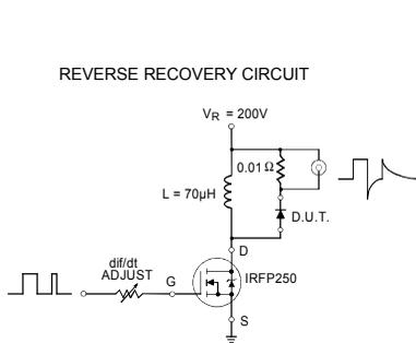
**Fig. 9** - Reverse Recovery Parameter Test Circuit
