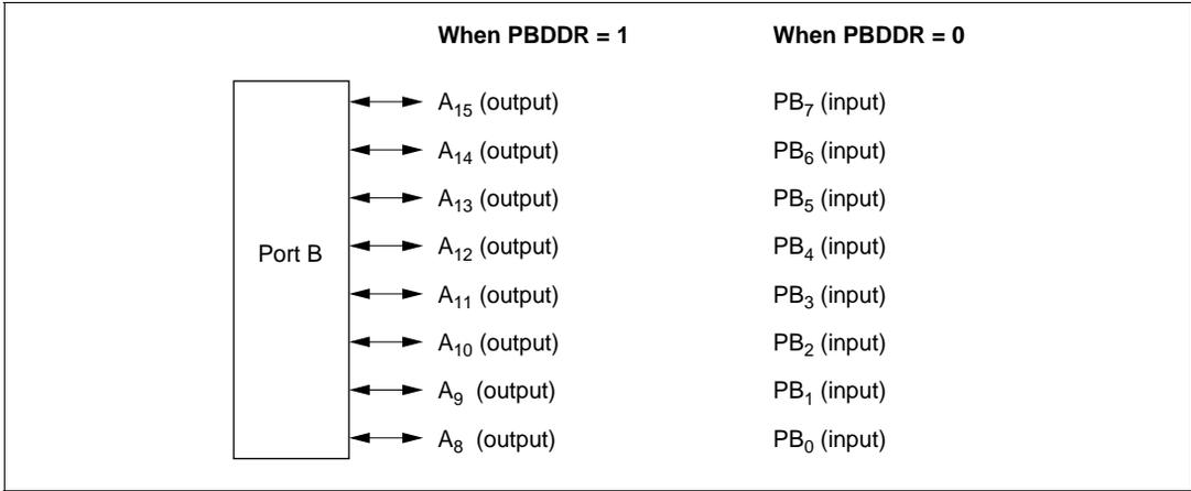
**Figure 5.13 Port B Pin Functions (Mode 6)**
