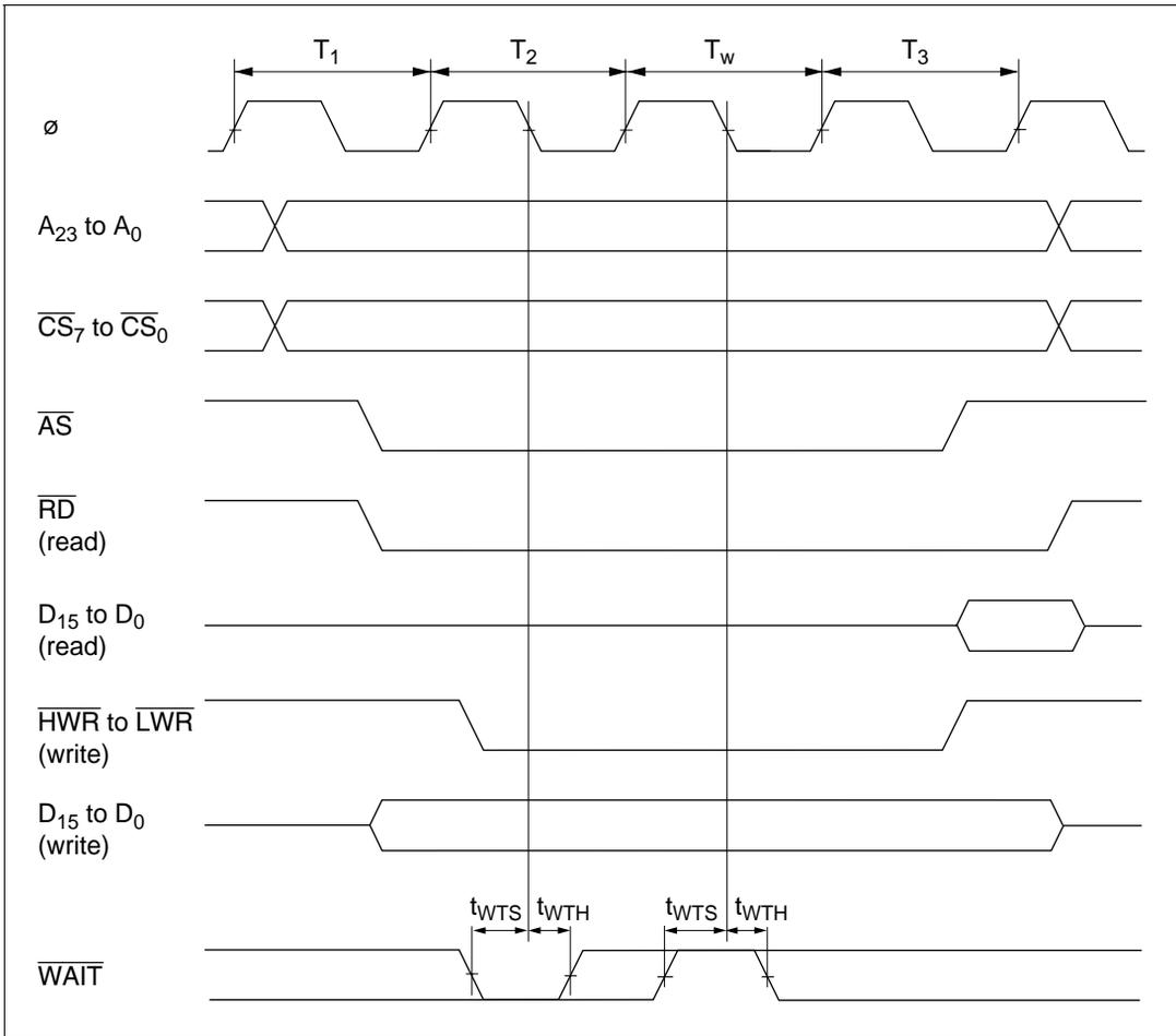
**Figure 7.8 Basic Bus Timing (3-State Access, 1 Wait)**
