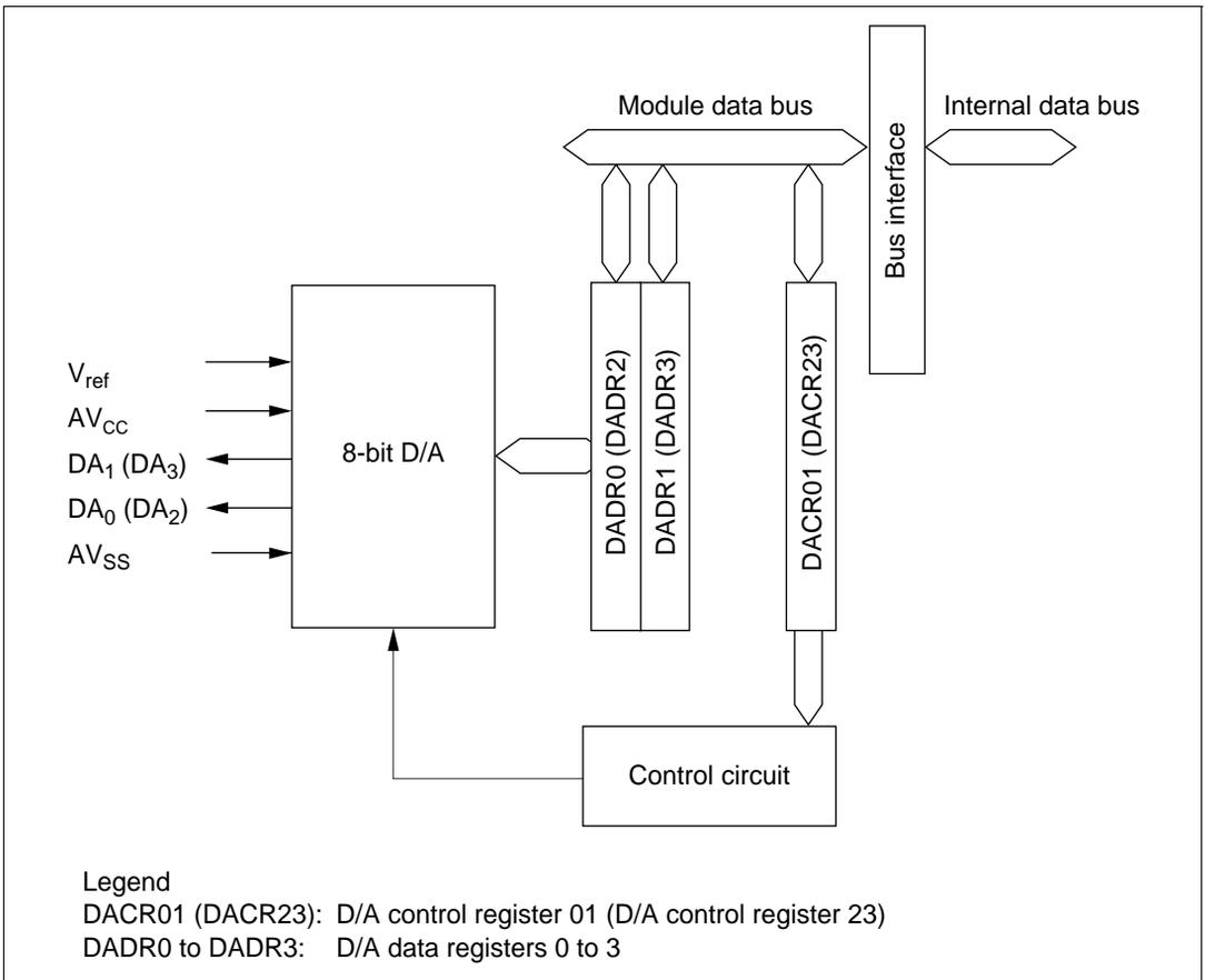
Figure 6.11 Block Diagram of D/A Converter
