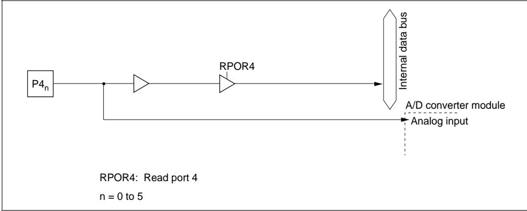
Figure 5.30 (a) Port 4 Block Diagram (Pins  $P4_0$  to  $P4_5$ )
