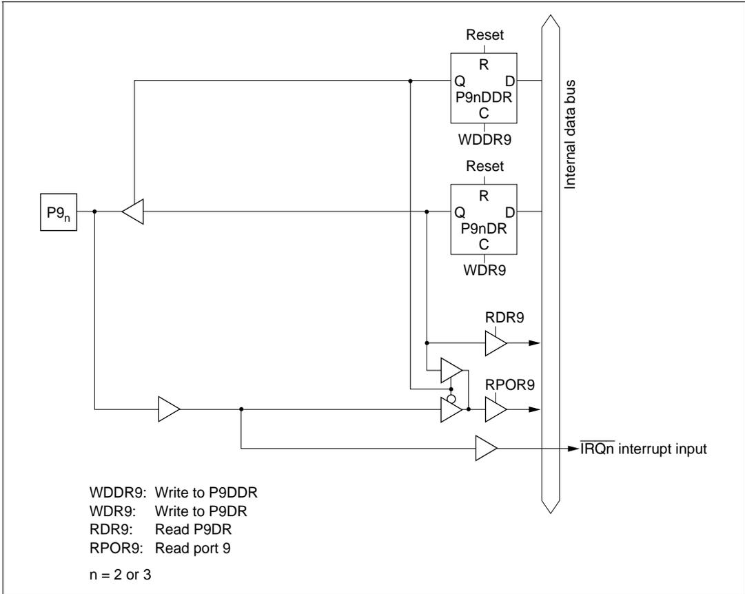
**Figure 5.35 (b) Port 9 Block Diagram (Pins  $P9_2$  and  $P9_3$ )**
