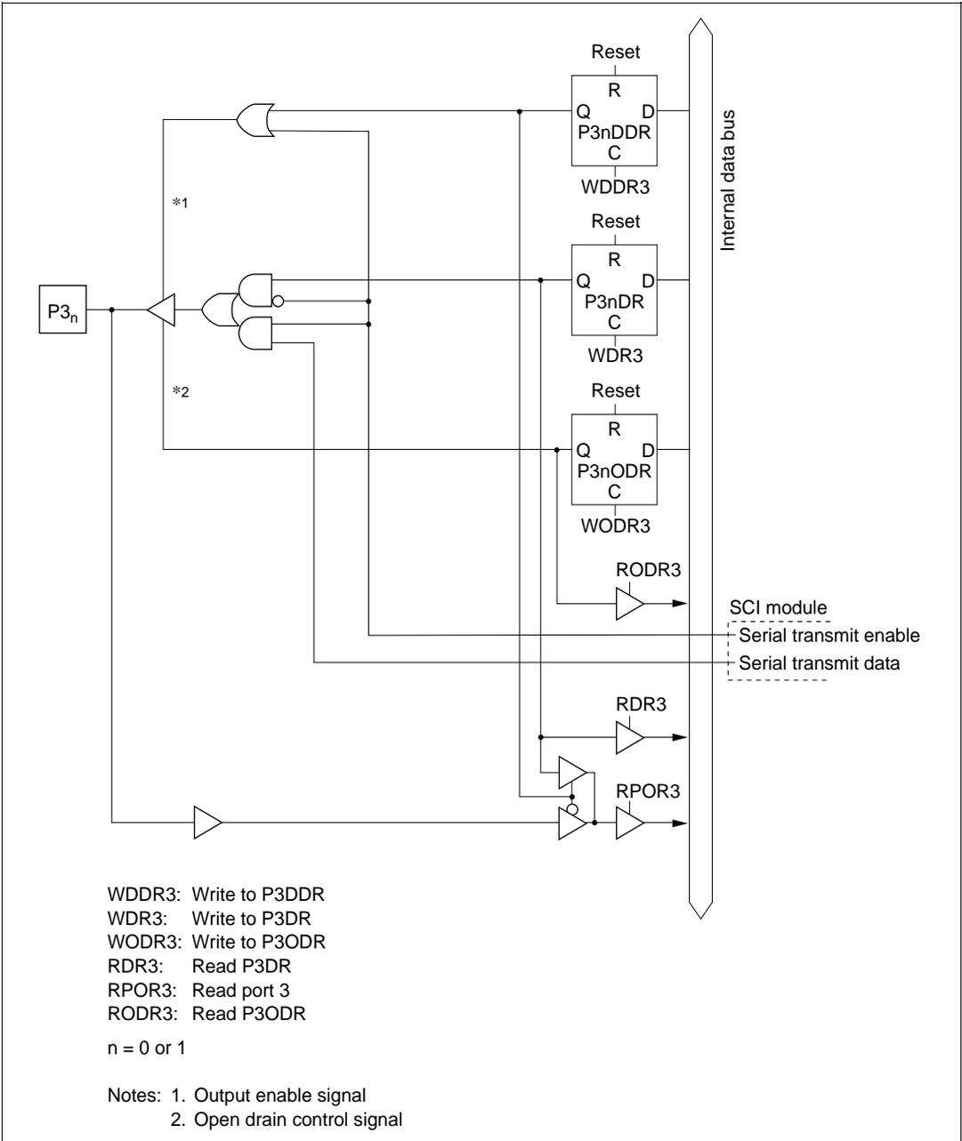
Figure 5.29 (a) Port 3 Block Diagram (Pins P3<sub>0</sub> and P3<sub>1</sub>)
