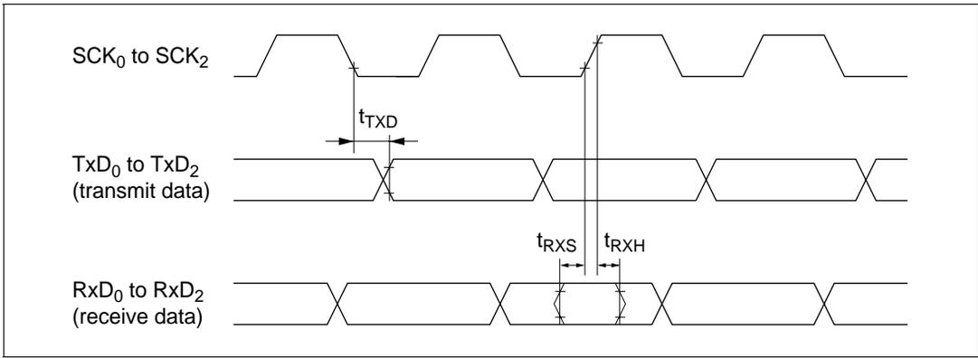
**Figure 7.29 SCI Input/Output Timing (Synchronous Mode)**
