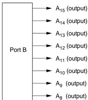
**Figure 5.12 Port B Pin Functions (Modes 4 and 5)**
