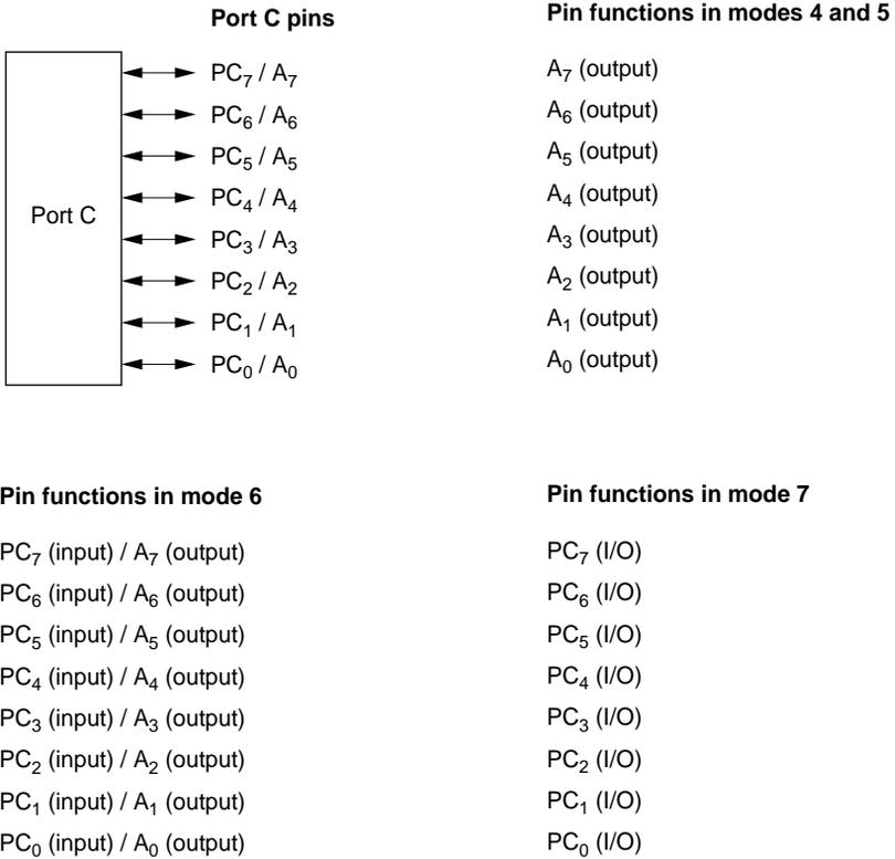
**Figure 5.15 Port C Pin Functions**
