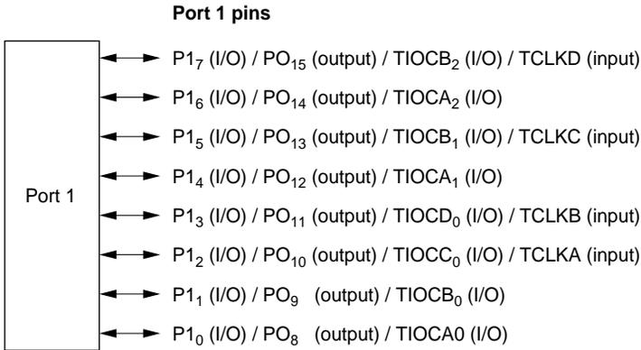
**Figure 5.1 Port 1 Pin Functions**
