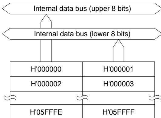
Figure 6.14 Block Diagram of Flash Memory (384 kbytes)
