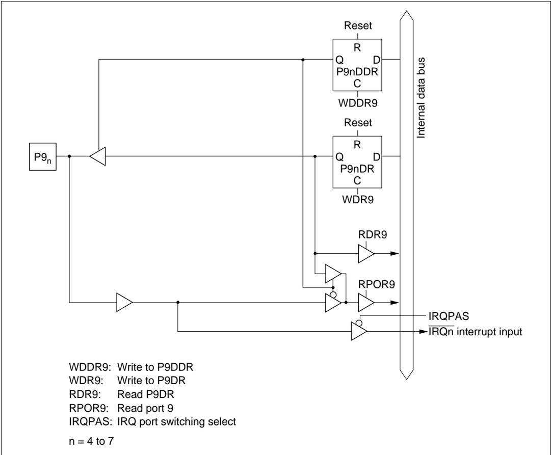
Figure 5.35 (a) Port 9 Block Diagram (Pins P9<sub>4</sub> to P9<sub>7</sub>)
