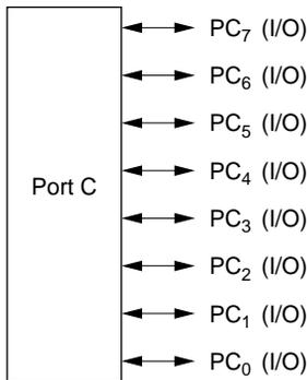
**Figure 5.18 Port C Pin Functions (Mode 7)**
