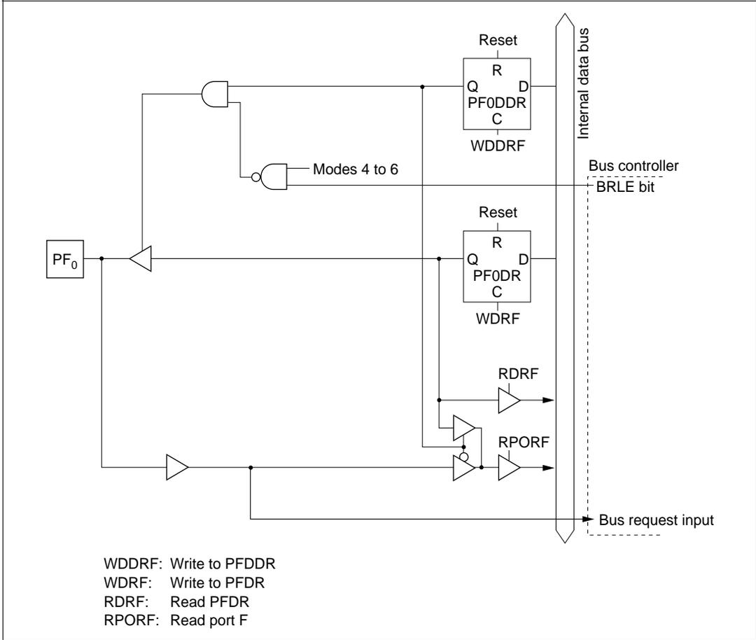
**Figure 5.41 (a) Port F Block Diagram (Pin PF<sub>0</sub>)**
