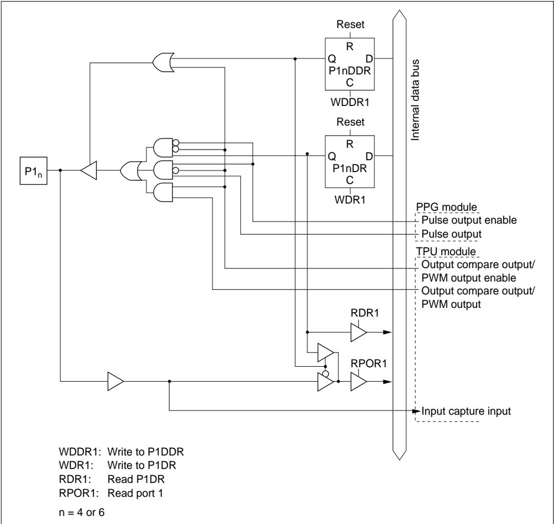
**Figure 5.27 (c) Port 1 Block Diagram (Pins P1<sub>4</sub> and P1<sub>6</sub>)**
