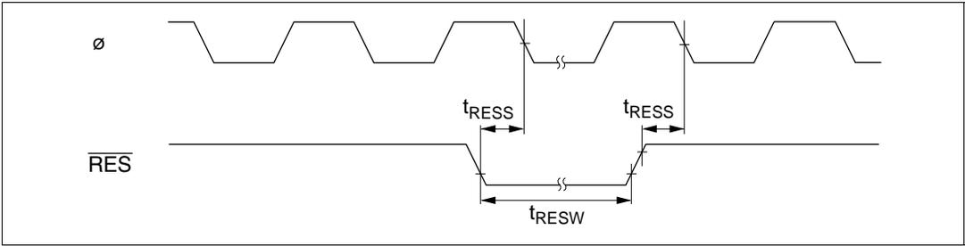
**Figure 7.4 Reset Input Timing**
