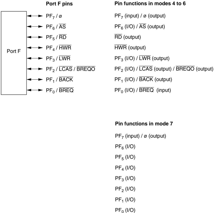
**Figure 5.25 Port F Pin Functions**
