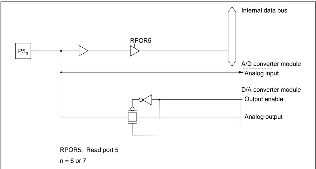
**Figure 5.31 (f) Port 5 Block Diagram (Pins P5<sub>6</sub> and P5<sub>7</sub>)**
