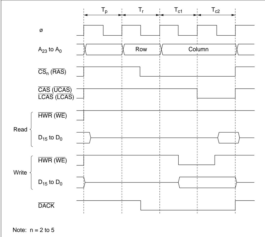
Figure 4.19  $\overline{\text{DACK}}$  Output Timing when DDS = 0 (Example of DRAM Access)
