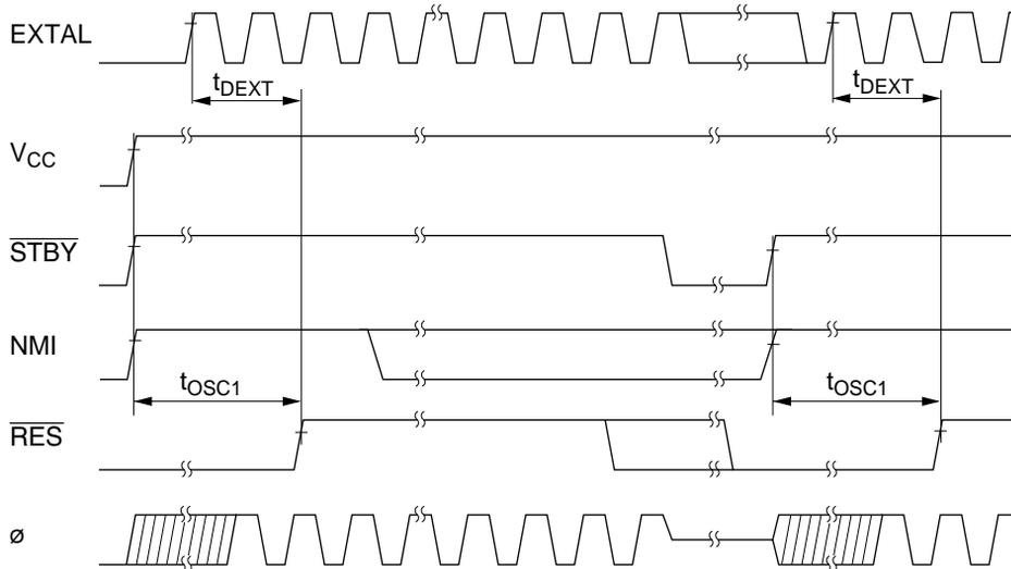
**Figure 7.3 Oscillation Stabilization Timing**
