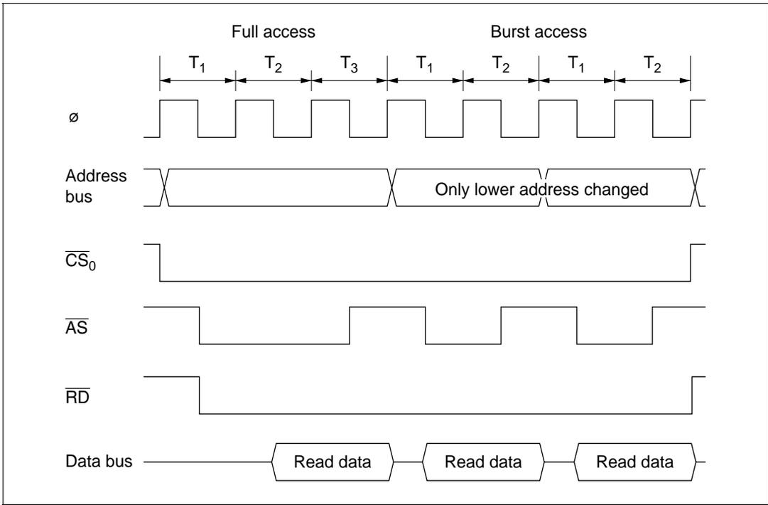
**Figure 4.20 (a) Example of Burst ROM Access Timing (When  $AST0 = BRSTS1 = 1$ )**
