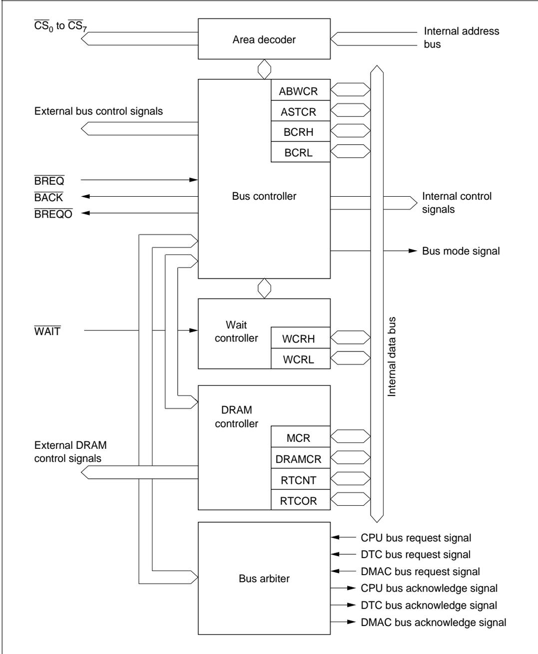
**Figure 4.1 Block Diagram of Bus Controller**
