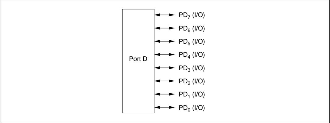
**Figure 5.21 Port D Pin Functions (Mode 7)**
