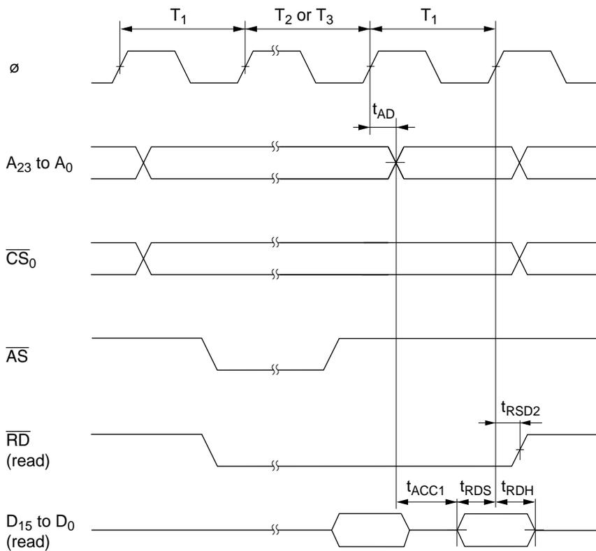
**Figure 7.13 Burst ROM Access Timing (1-State Access)**
