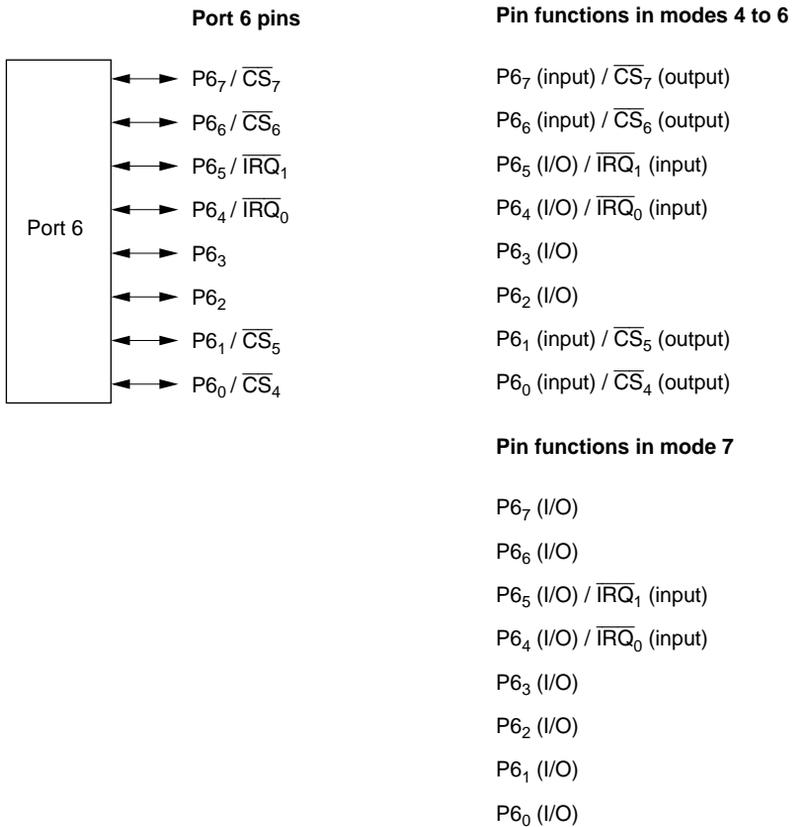
Figure 5.6 Port 6 Pin Functions
