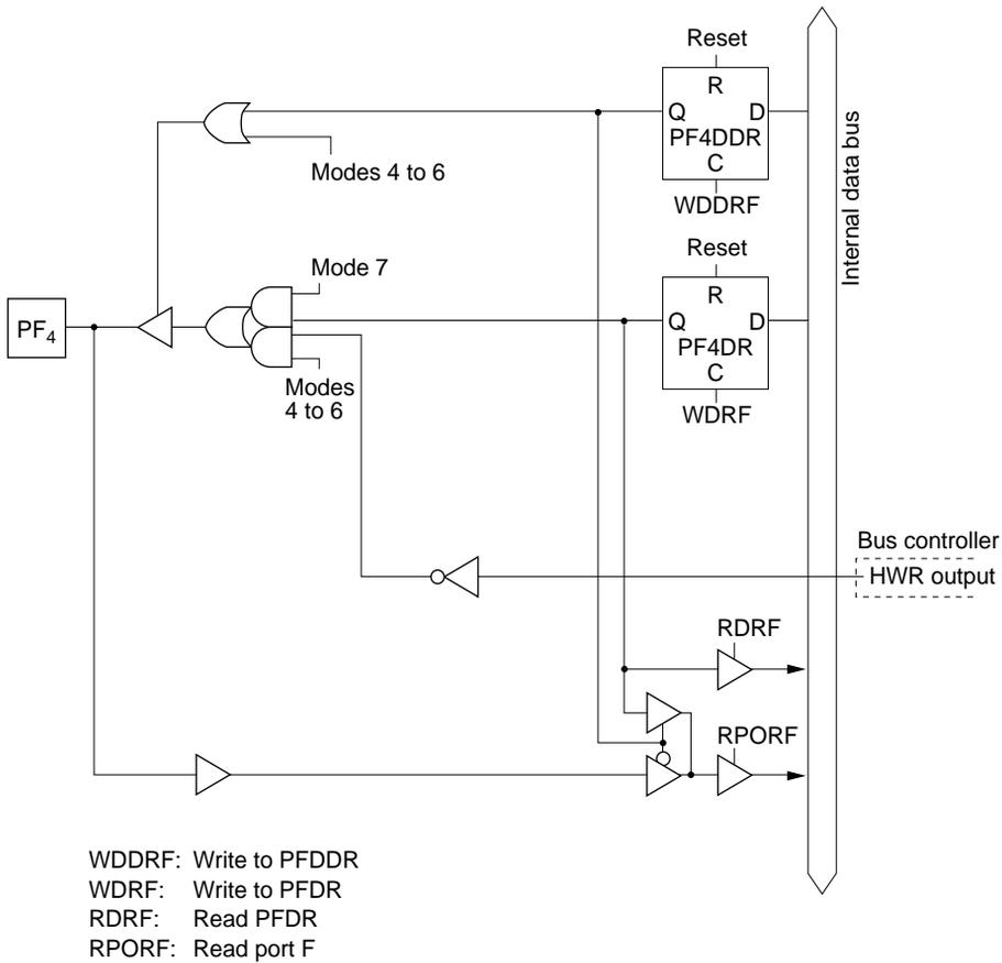
**Figure 5.41 (e) Port F Block Diagram (Pin PF<sub>4</sub>)**
