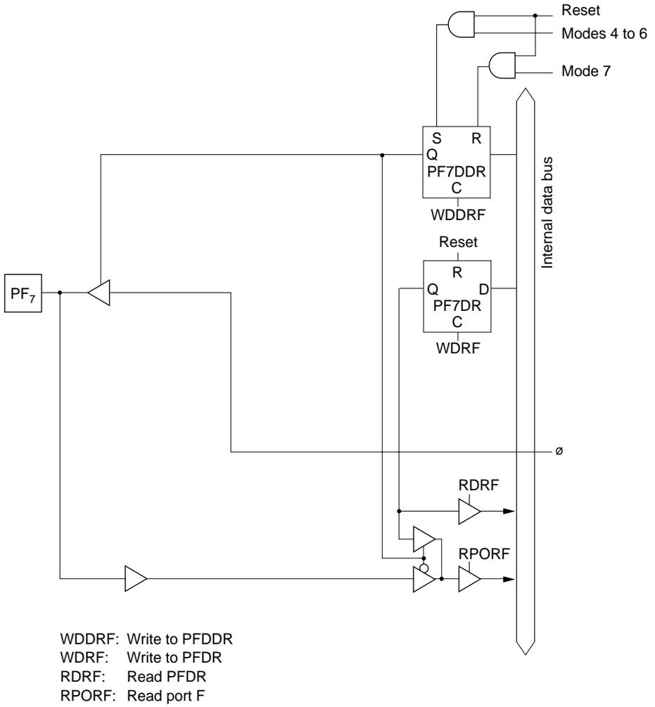
**Figure 5.41 (h) Port F Block Diagram (Pin PF<sub>7</sub>)**
