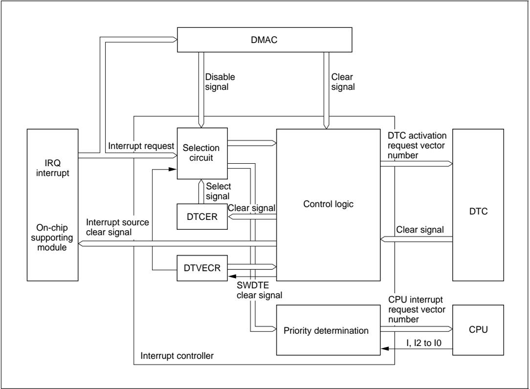
Figure 3.3 Interrupt Control for DTC and DMAC
