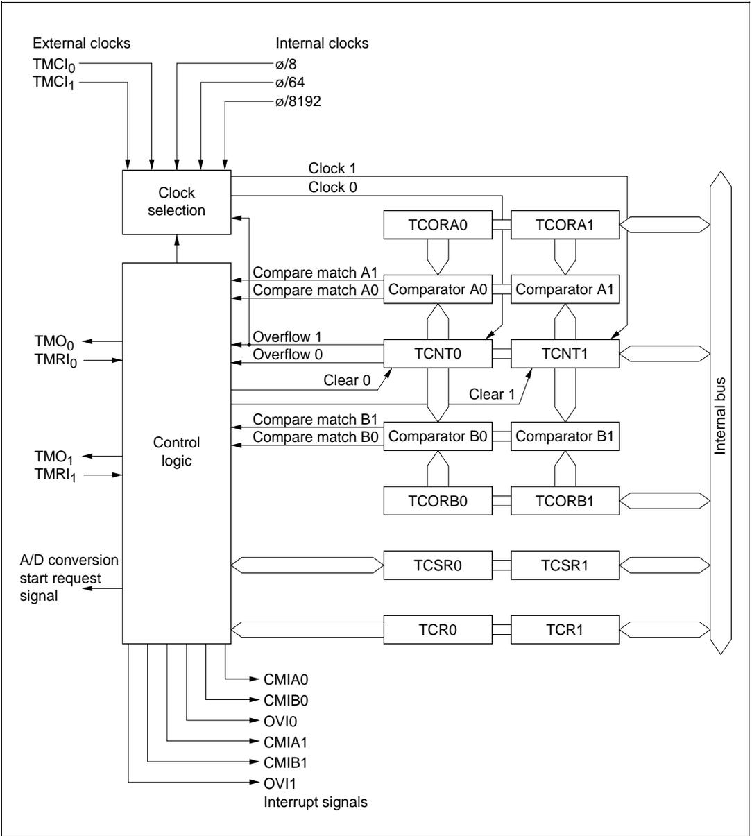
Figure 6.6 Block Diagram of 8-Bit Timer
