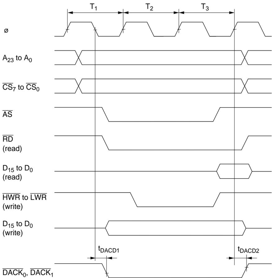
**Figure 7.17 DMAC Single Address Transfer Timing (3-State Access)**
