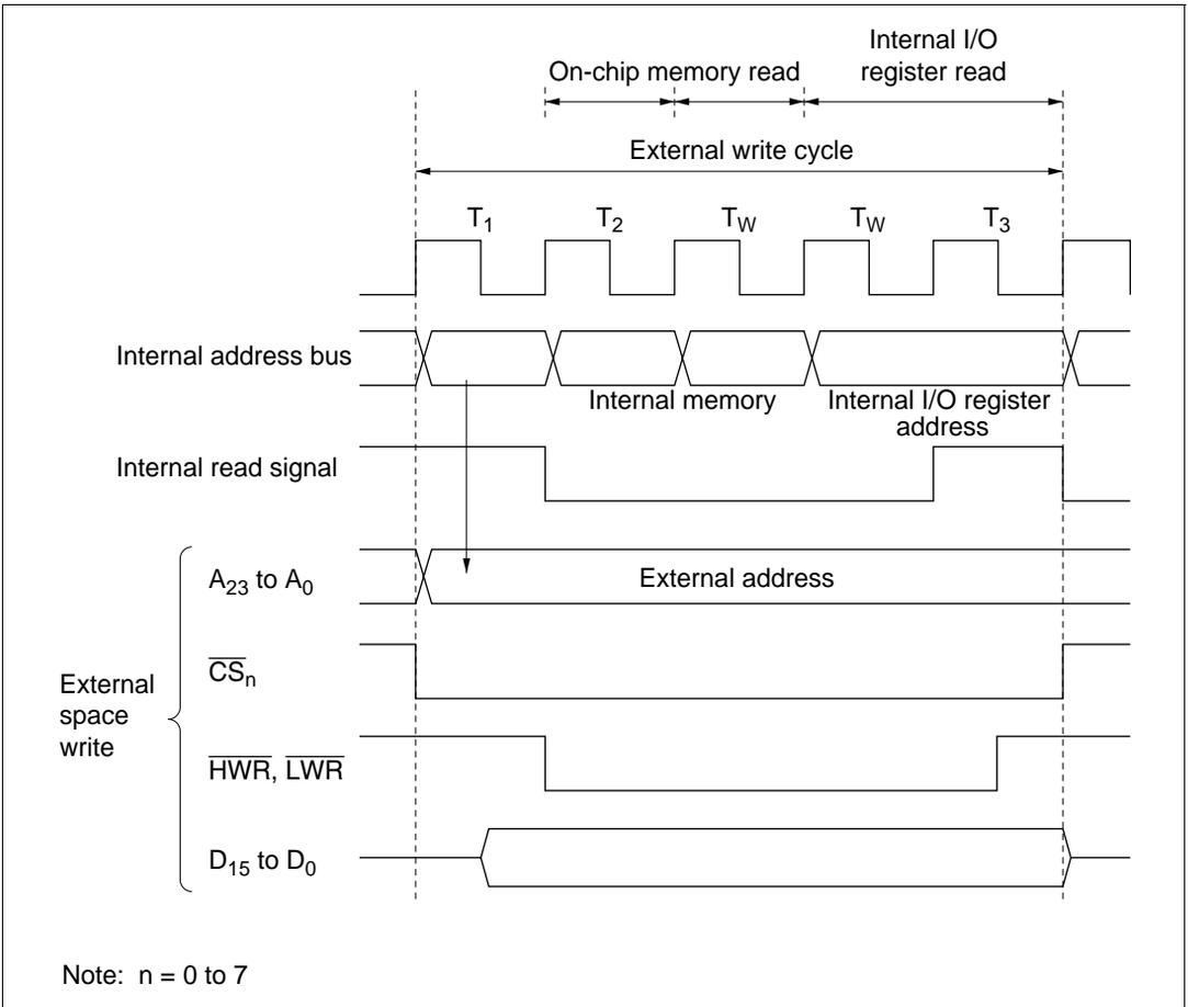
**Figure 4.26 Example of Timing when Write Data Buffer Function is Used**
