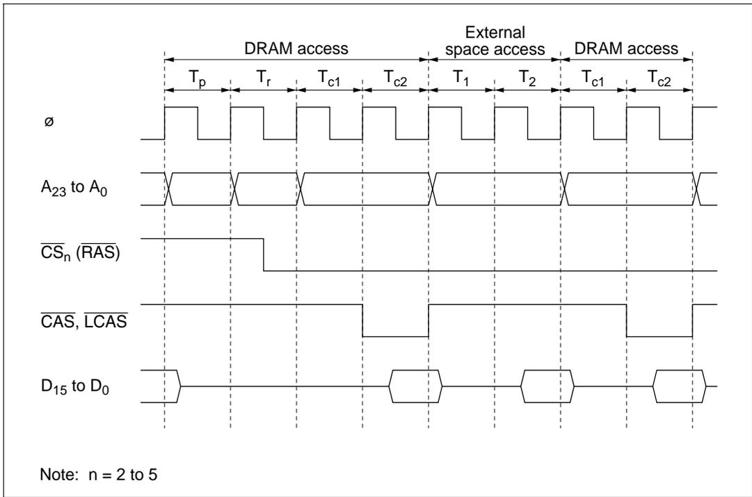
**Figure 4.11 Example of Operation Timing in RAS Down Mode**
