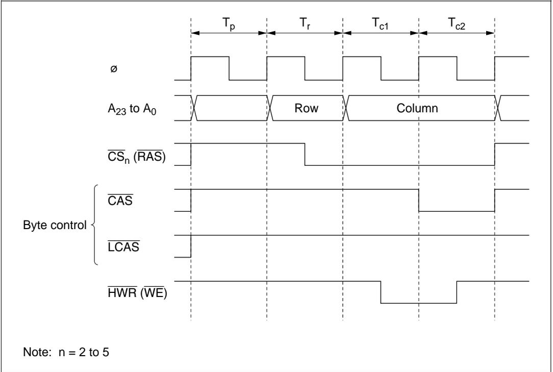
**Figure 4.8 2-CAS Control Timing (Upper Byte Write Access)**
