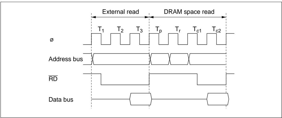
**Figure 4.24 Example of DRAM Access after External Read**
