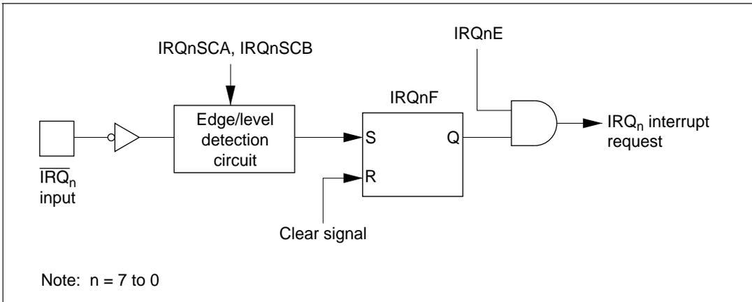
Figure 3.1 Block Diagram of Interrupts  $IRQ_7$  to  $IRQ_0$
