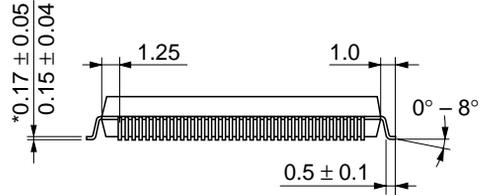
\*Dimension including the plating thickness
