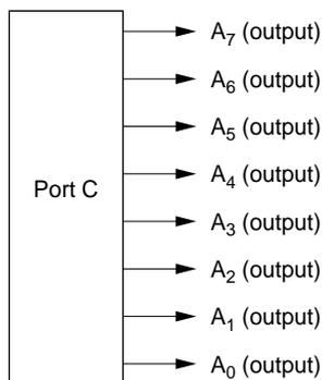
**Figure 5.16 Port C Pin Functions (Modes 4 and 5)**
