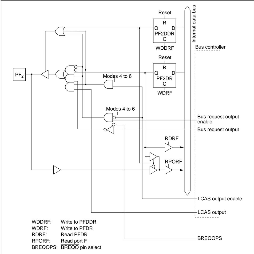
**Figure 5.41 (c) Port F Block Diagram (Pin PF<sub>2</sub>)**
