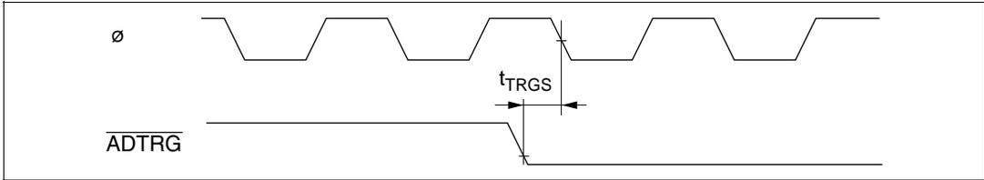
**Figure 7.30 A/D Converter External Trigger Input Timing**
