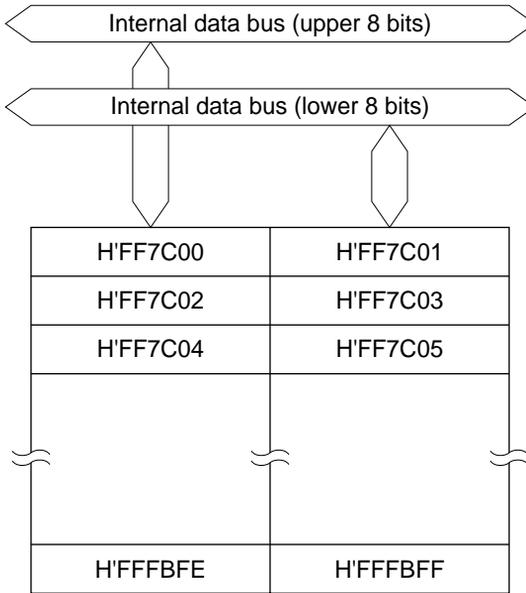
Figure 6.12 Block Diagram of RAM (32 kbytes)
