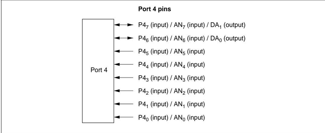
**Figure 5.4 Port 4 Pin Functions**
