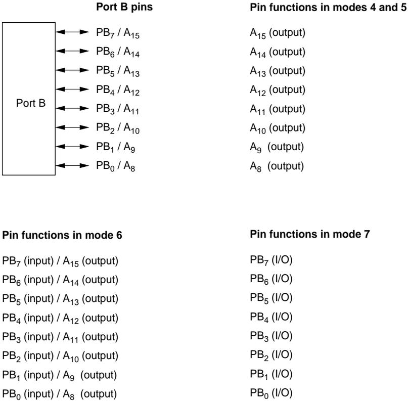
**Figure 5.11 Port B Pin Functions**
