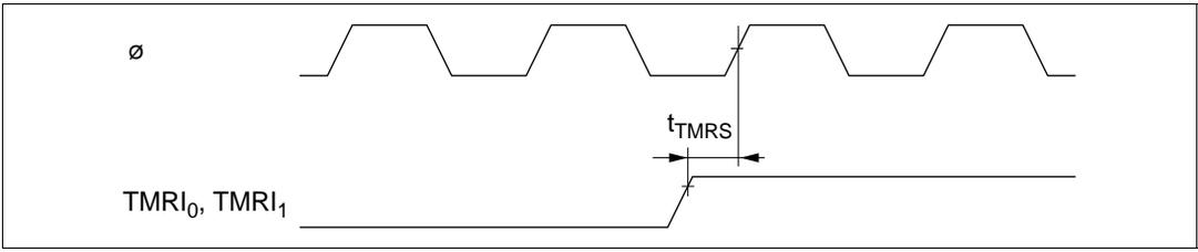
**Figure 7.26 8-Bit Timer Reset Input Timing**
