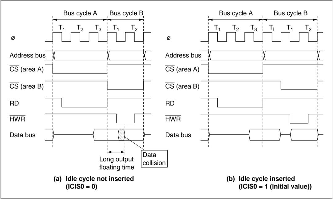
**Figure 4.22 Example of Idle Cycle Operation (2)**
