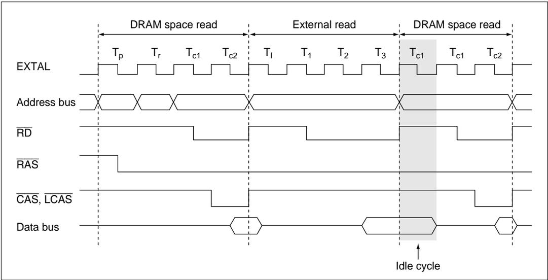
**Figure 4.25 (a) Example of Idle Cycle Insertion in RAS Down Mode (ICIS1 = 1)**
