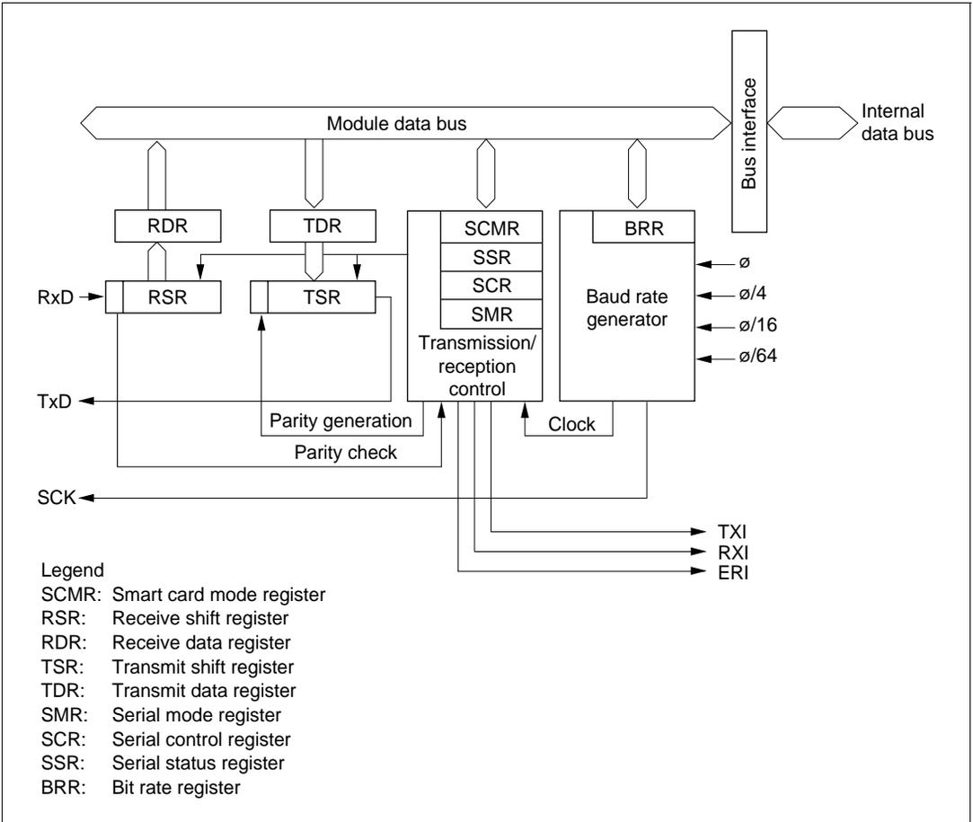
Figure 6.9 Block Diagram of Smart Card Interface
