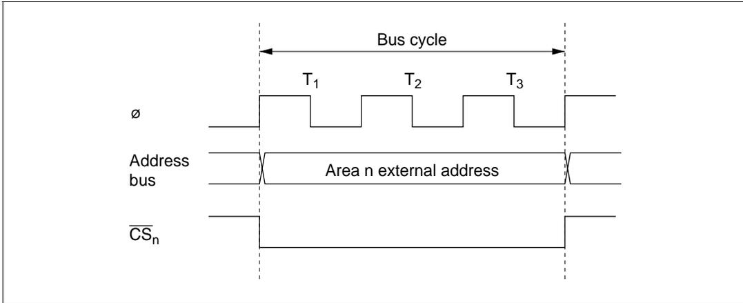
Figure 4.3  $\overline{CS}_n$  Signal Output Timing ( $n = 0$  to  $7$ )
