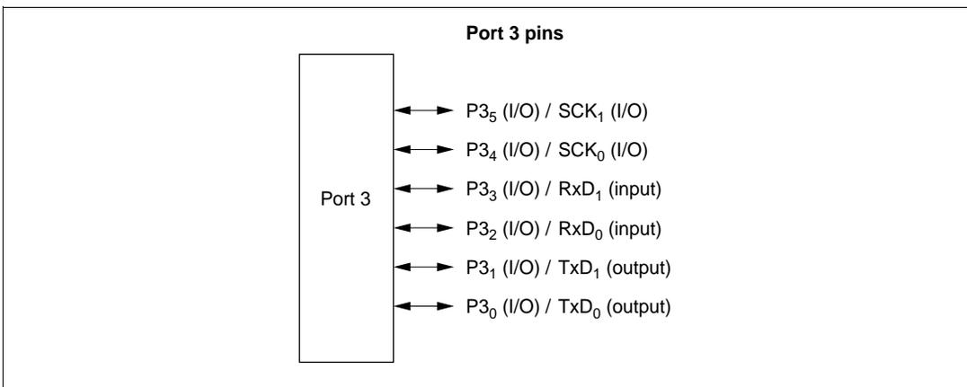
**Figure 5.3 Port 3 Pin Functions**
