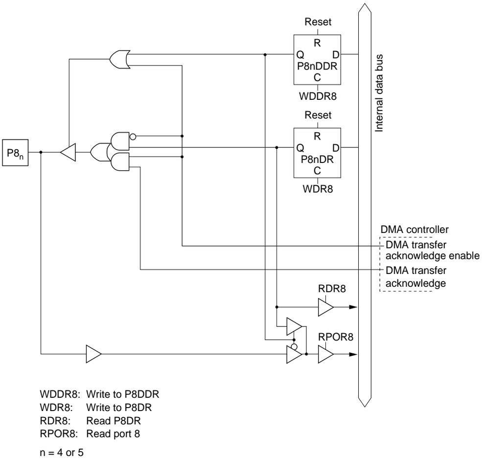
**Figure 5.34 (c) Port 8 Block Diagram (Pins  $P8_4$  and  $P8_5$ )**
