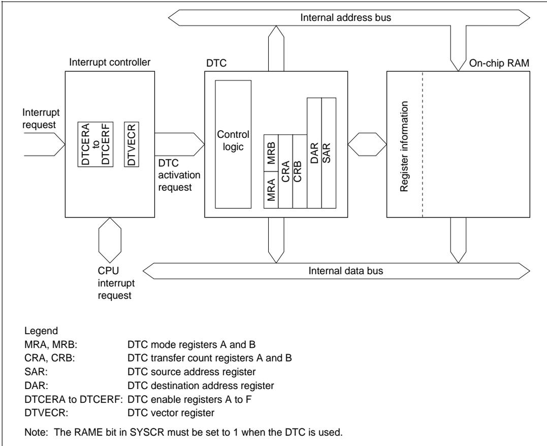
**Figure 6.3 Block Diagram of DTC**
