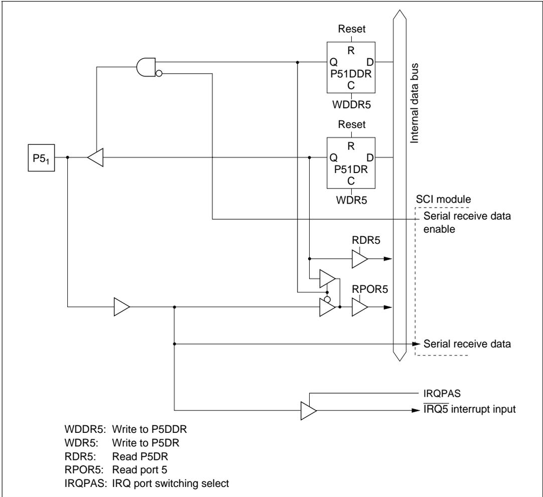
**Figure 5.31 (b) Port 5 Block Diagram (Pin P5<sub>1</sub>)**
