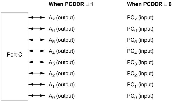
**Figure 5.17 Port C Pin Functions (Mode 6)**
