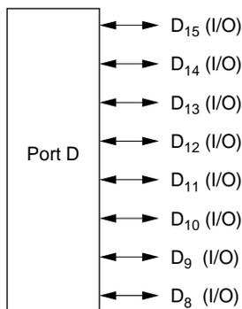
**Figure 5.20 Port D Pin Functions (Modes 4 to 6)**
