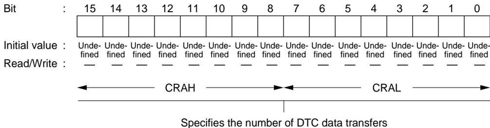
**CRB—DTC Transfer Count Register B****H'F800—H'FBFF****DTC**
