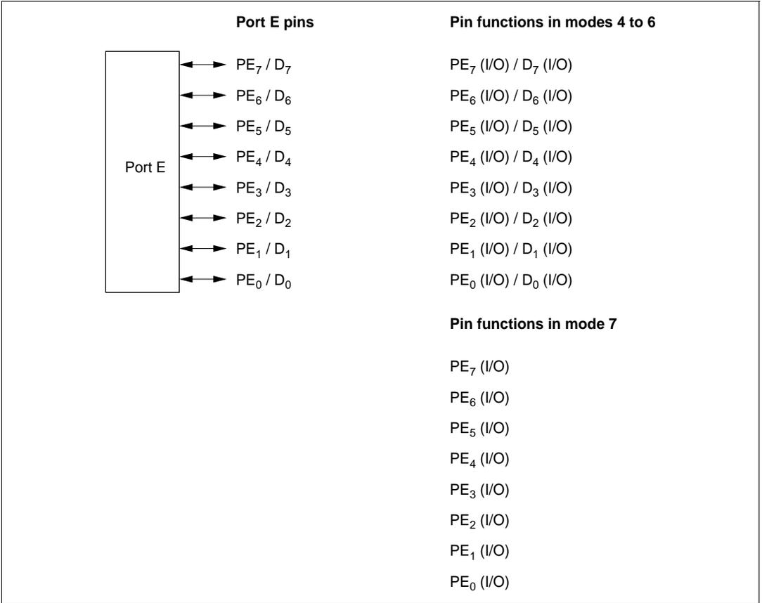
**Figure 5.22 Port E Pin Functions**
