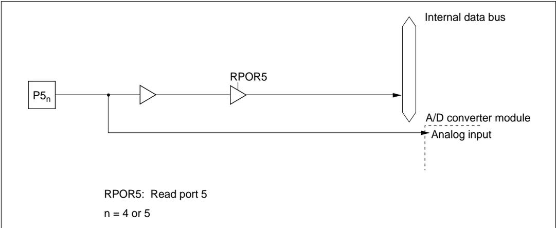
**Figure 5.31 (e) Port 5 Block Diagram (Pins P5<sub>4</sub> and P5<sub>5</sub>)**
