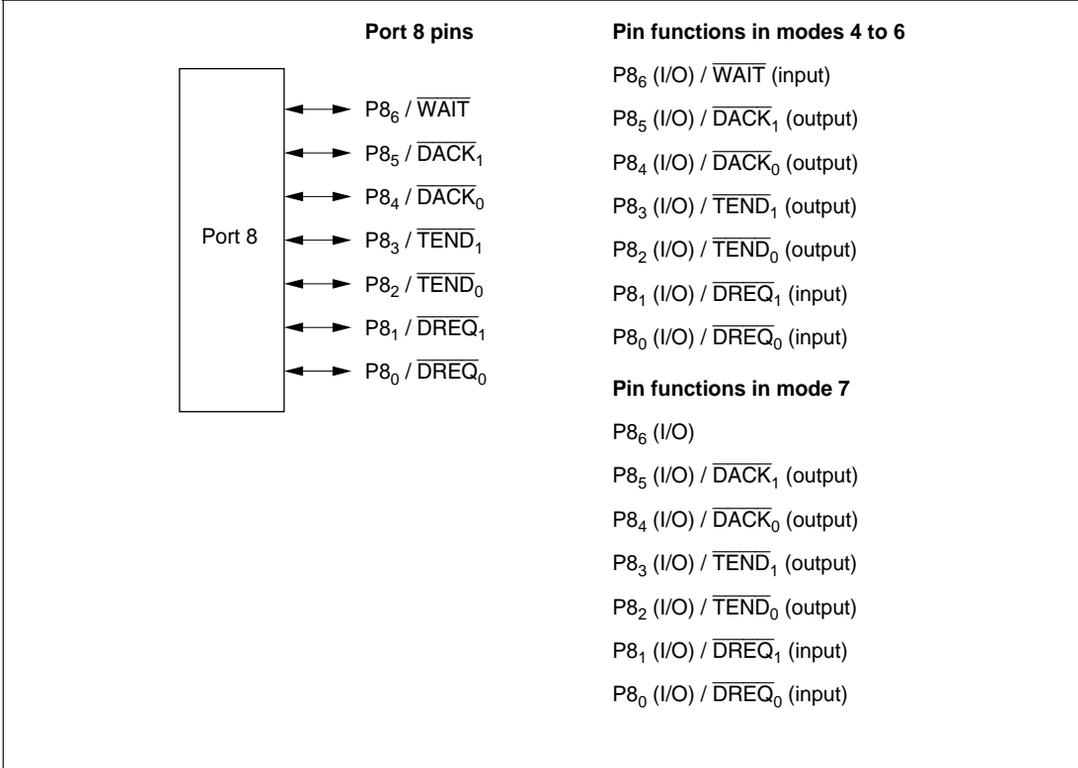
Figure 5.8 Port 8 Pin Functions
