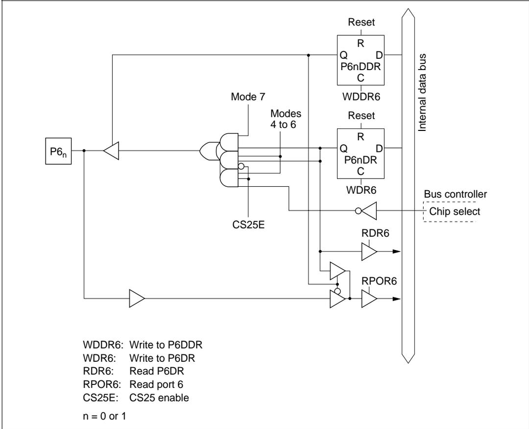
Figure 5.32 (a) Port 6 Block Diagram (Pins  $P6_0$  and  $P6_1$ )
