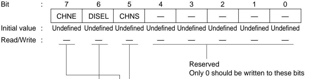
**DTC Chain Transfer Enable, DTC Chain Transfer Select**
