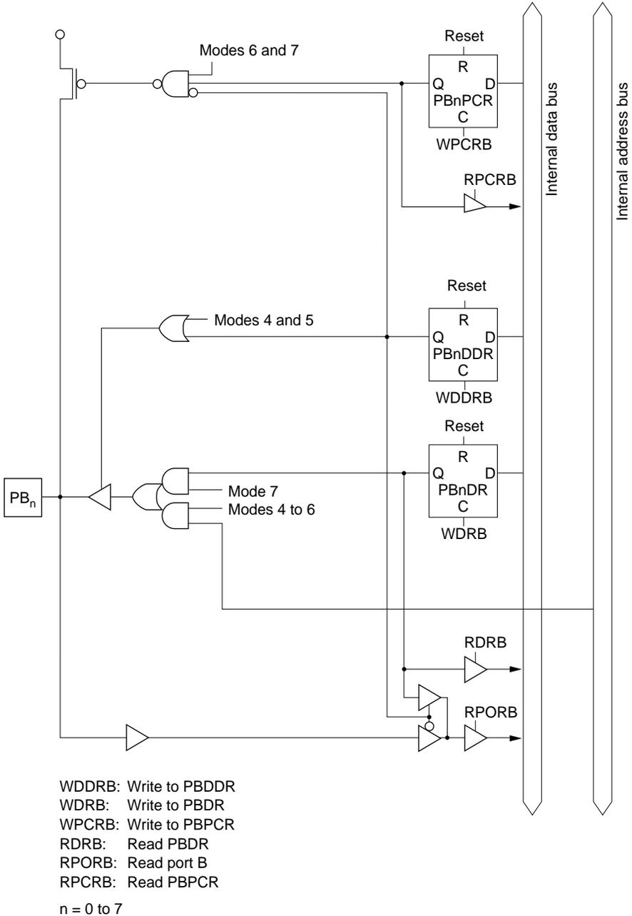
Figure 5.37 Port B Block Diagram (Pins PB<sub>n</sub>)
