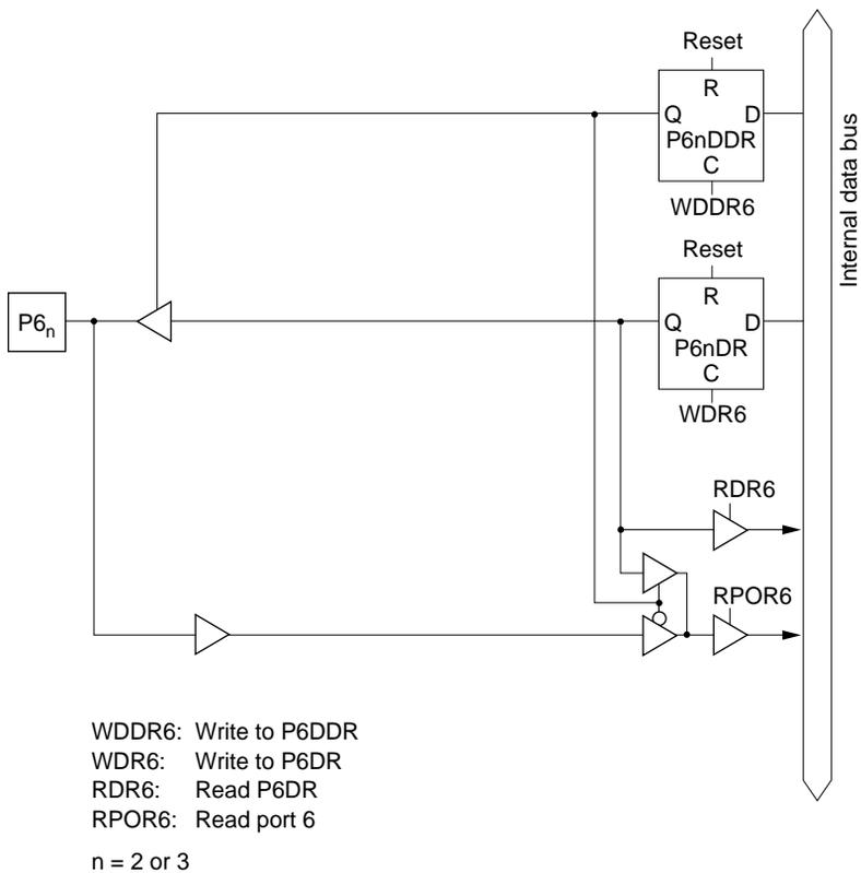
**Figure 5.32 (b) Port 6 Block Diagram (Pins  $P6_2$  and  $P6_3$ )**
