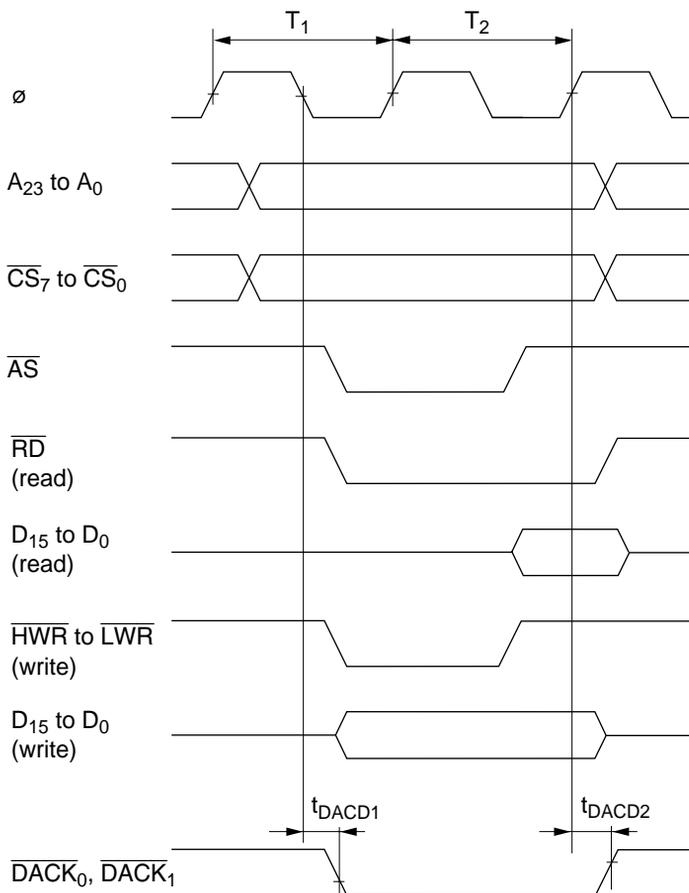
**Figure 7.16 DMAC Single Address Transfer Timing (2-State Access)**
