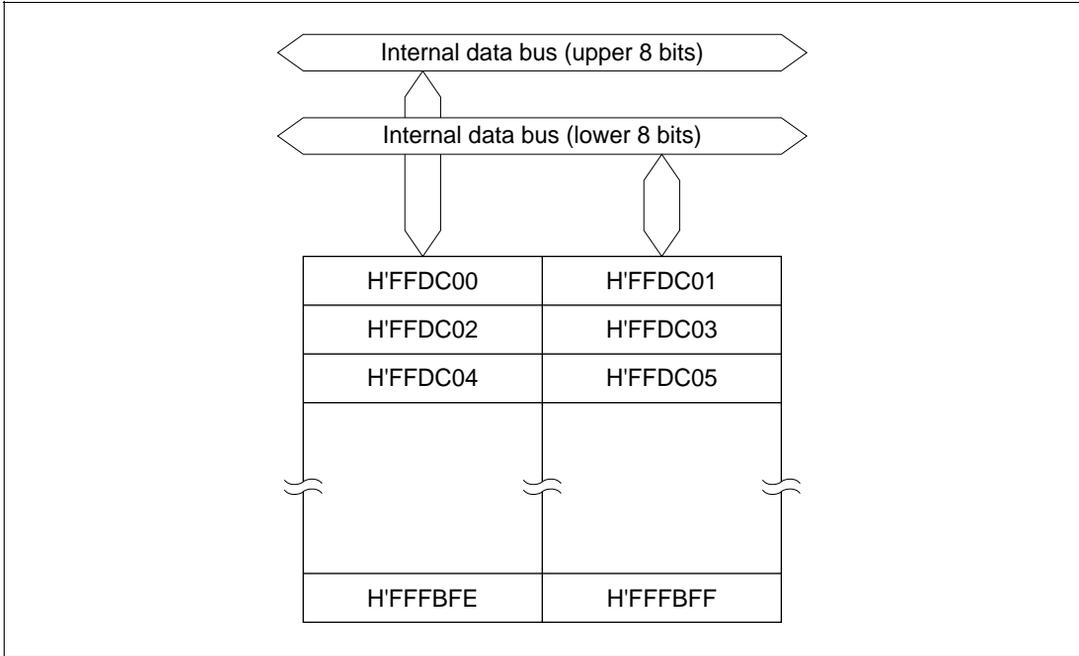
**Figure 6.13 Block Diagram of RAM (8 kbytes)**
