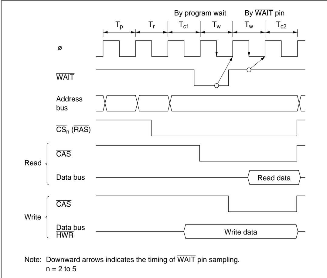
Figure 4.7 Example of Wait State Insertion Timing
