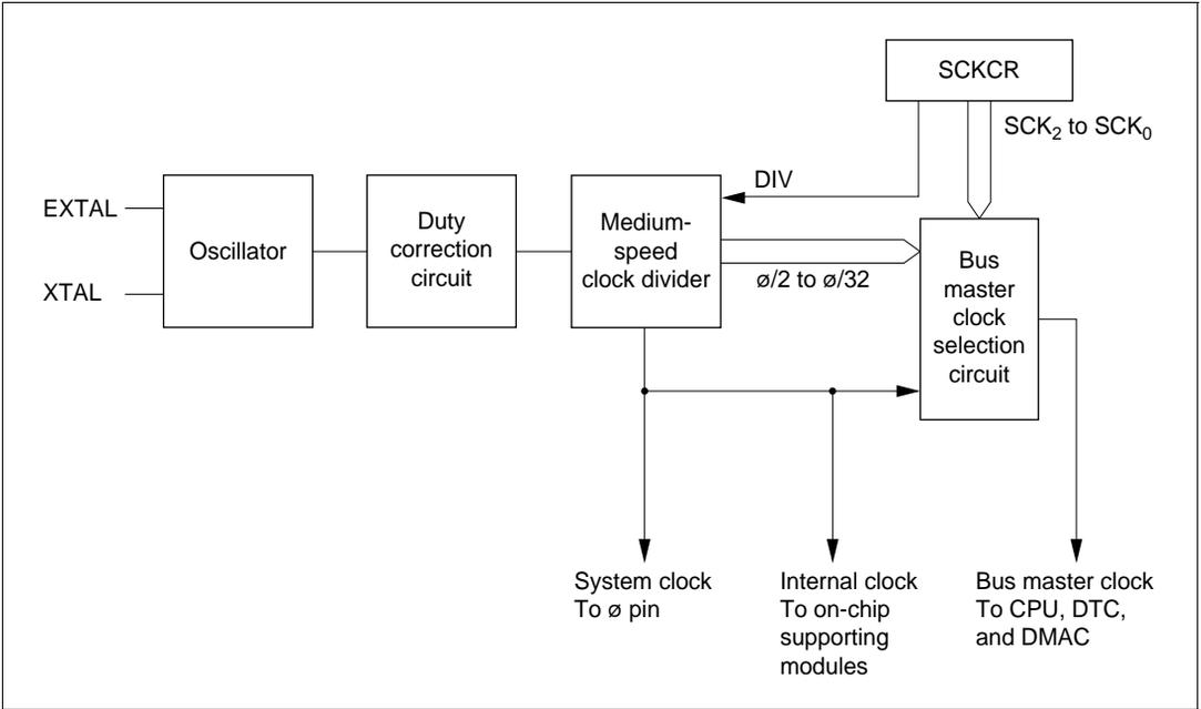
Figure 6.18 Block Diagram of Clock Pulse Generator
