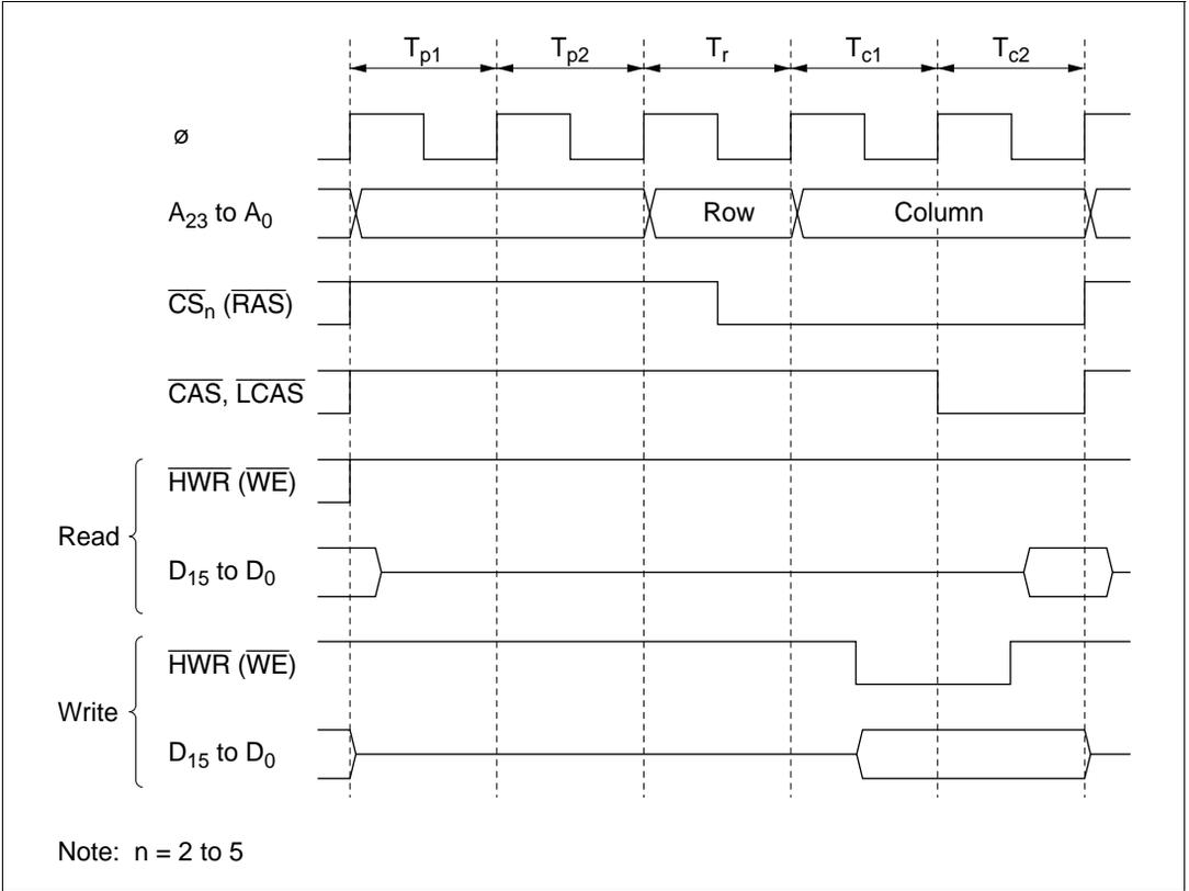
Figure 4.6 Timing with Two-State Precharge Cycle
