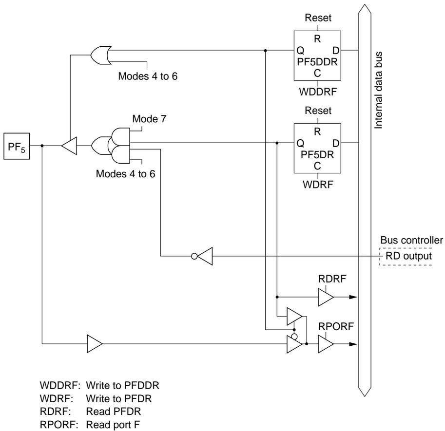
**Figure 5.41 (f) Port F Block Diagram (Pin PF<sub>5</sub>)**
