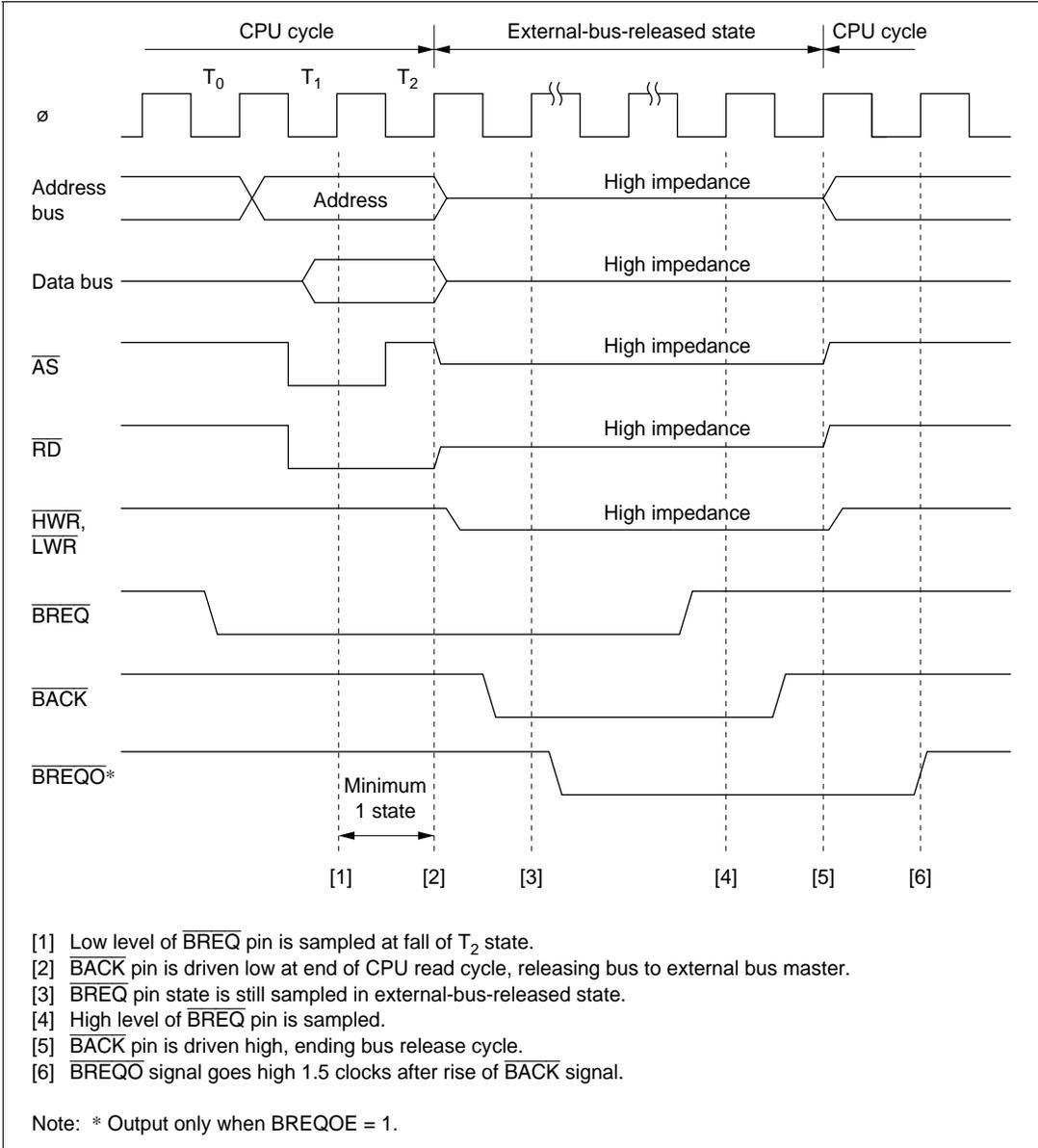
**Figure 4.27 Bus-Released State Transition Timing**
