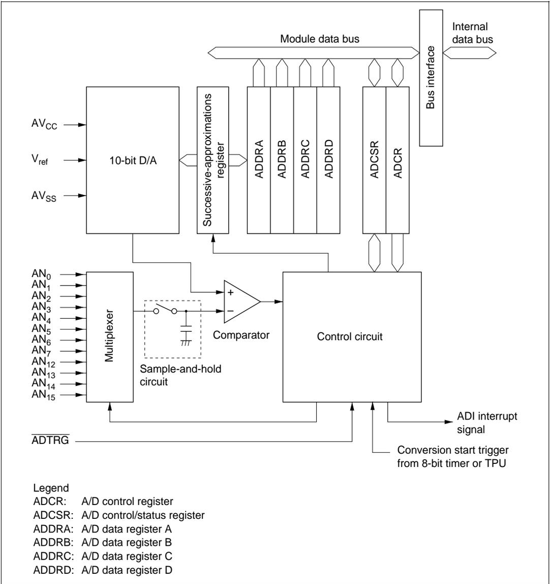
Figure 6.10 Block Diagram of A/D Converter
