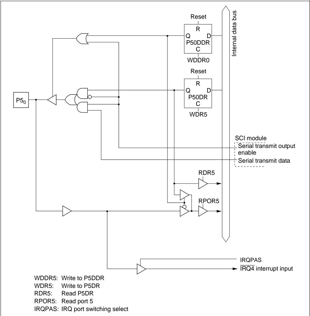
Figure 5.31 (a) Port 5 Block Diagram (Pin P5<sub>0</sub>)
