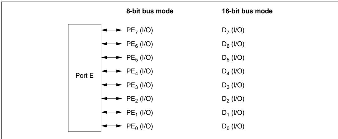
**Figure 5.23 Port E Pin Functions (Modes 4 to 6)**
