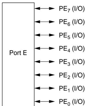
**Figure 5.24 Port E Pin Functions (Mode 7)**
