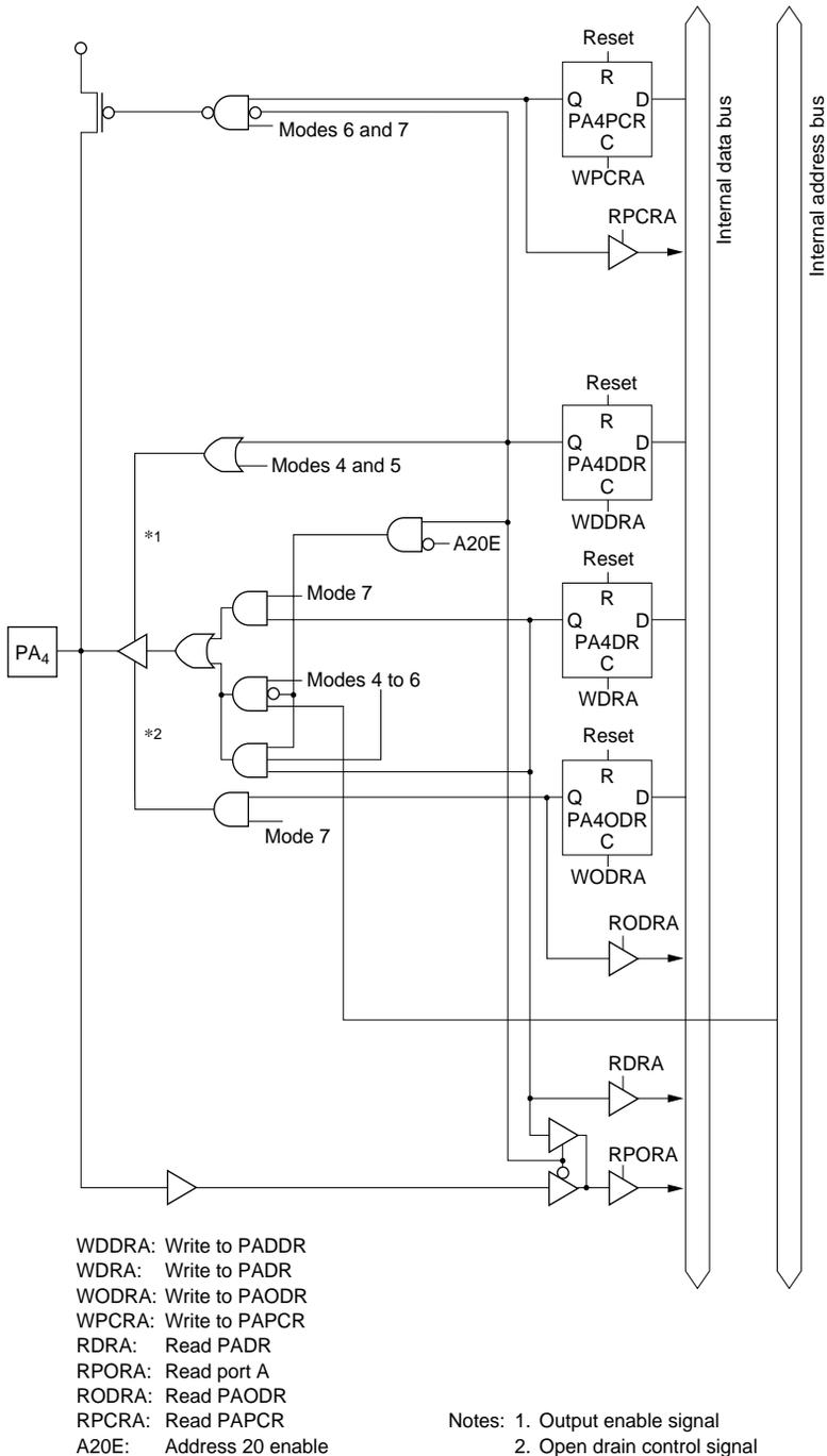
**Figure 5.36 (b) Port A Block Diagram (Pin PA<sub>4</sub>)**
