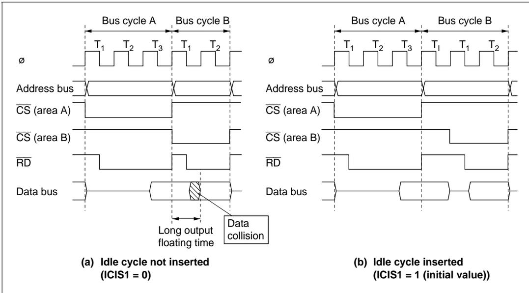
Figure 4.21 Example of Idle Cycle Operation (1)
