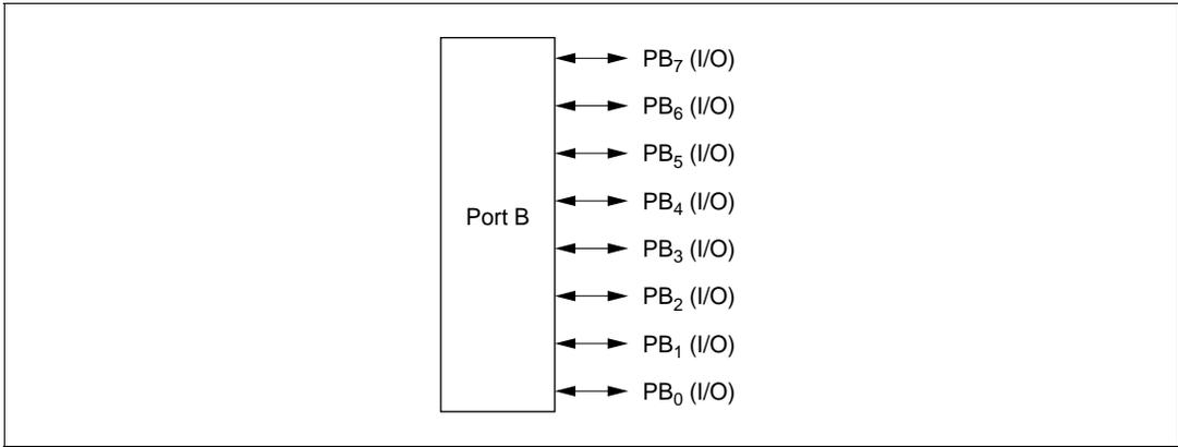
**Figure 5.14 Port B Pin Functions (Mode 7)**
