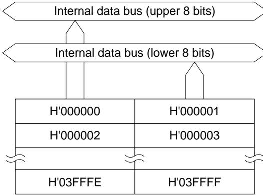
**Figure 6.16** Block Diagram of Flash Memory (256 kbytes)
