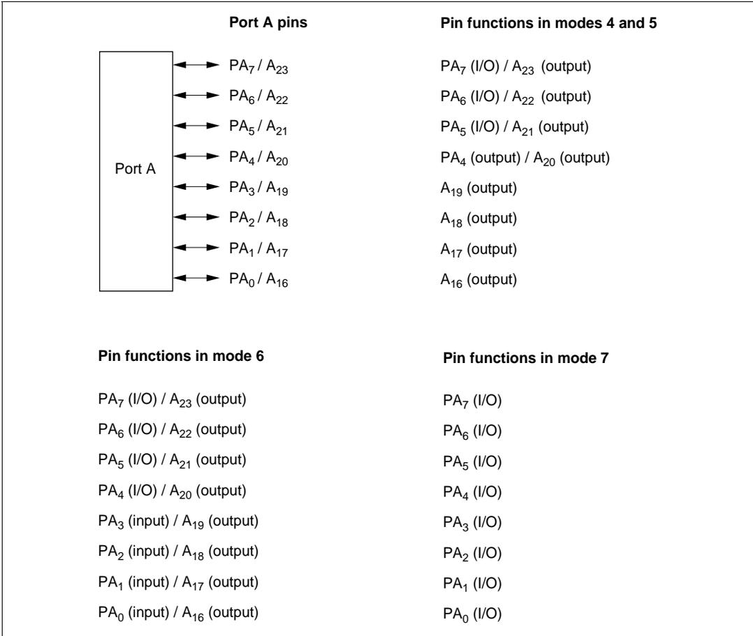
**Figure 5.10 Port A Pin Functions**
