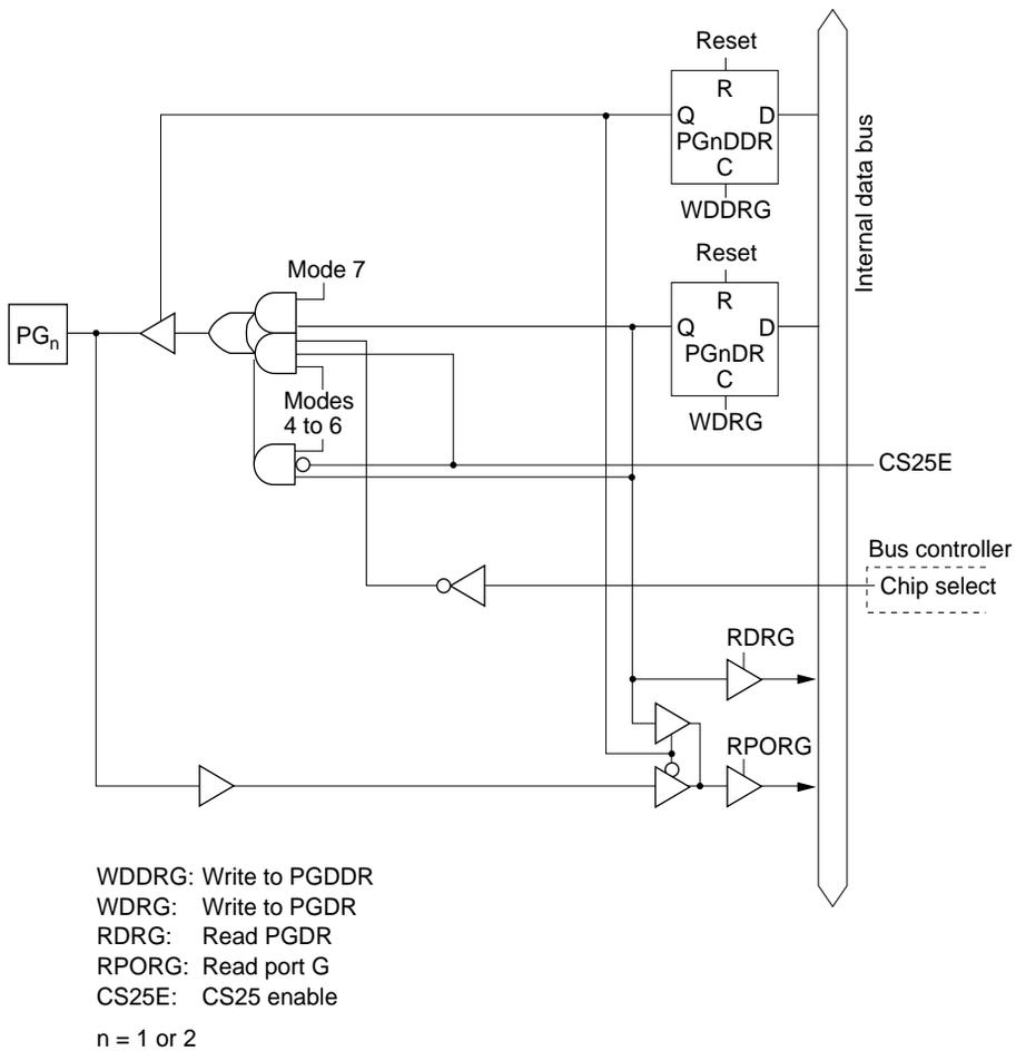
**Figure 5.42 (b) Port G Block Diagram (Pins PG<sub>1</sub> and PG<sub>2</sub>)**
