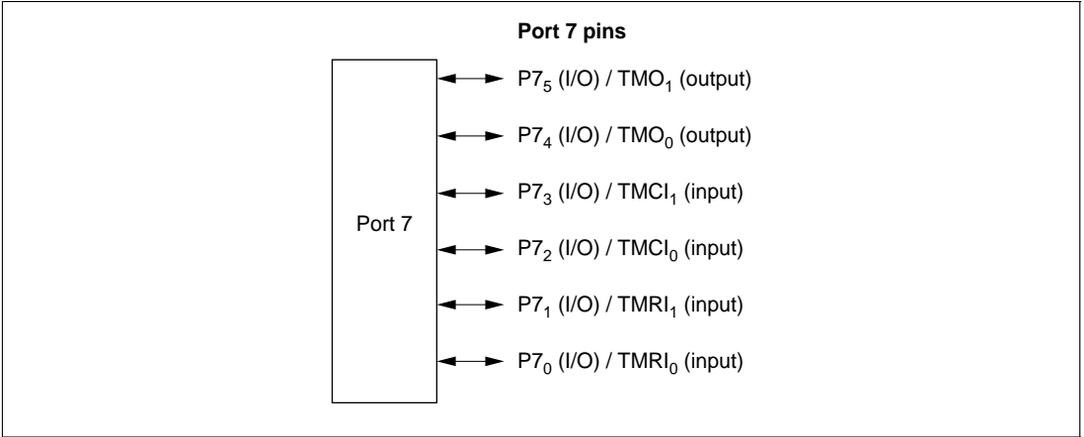
**Figure 5.7 Port 7 Pin Functions**
