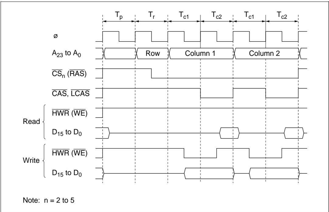
**Figure 4.10 Operation Timing in Fast Page Mode**
