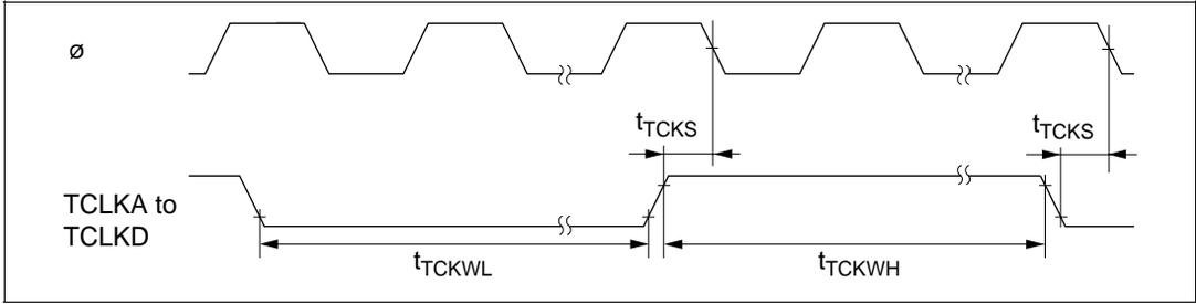
**Figure 7.23 TPU Clock Input Timing**
