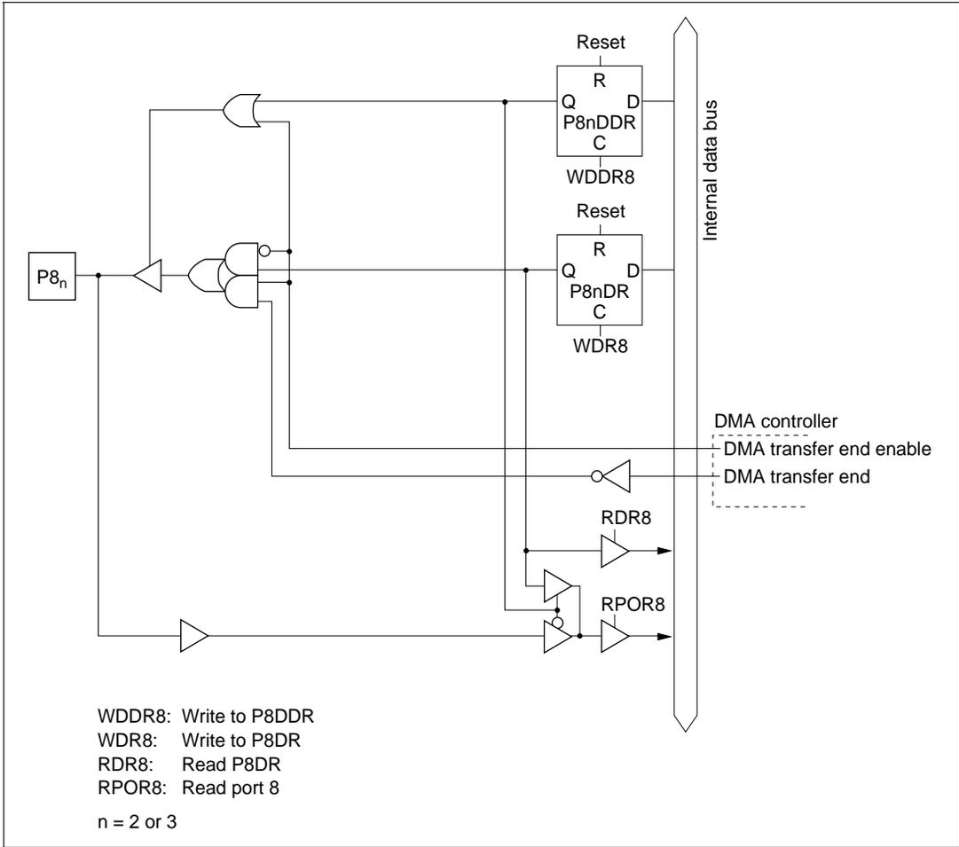
**Figure 5.34 (b) Port 8 Block Diagram (Pins  $P8_2$  and  $P8_3$ )**
