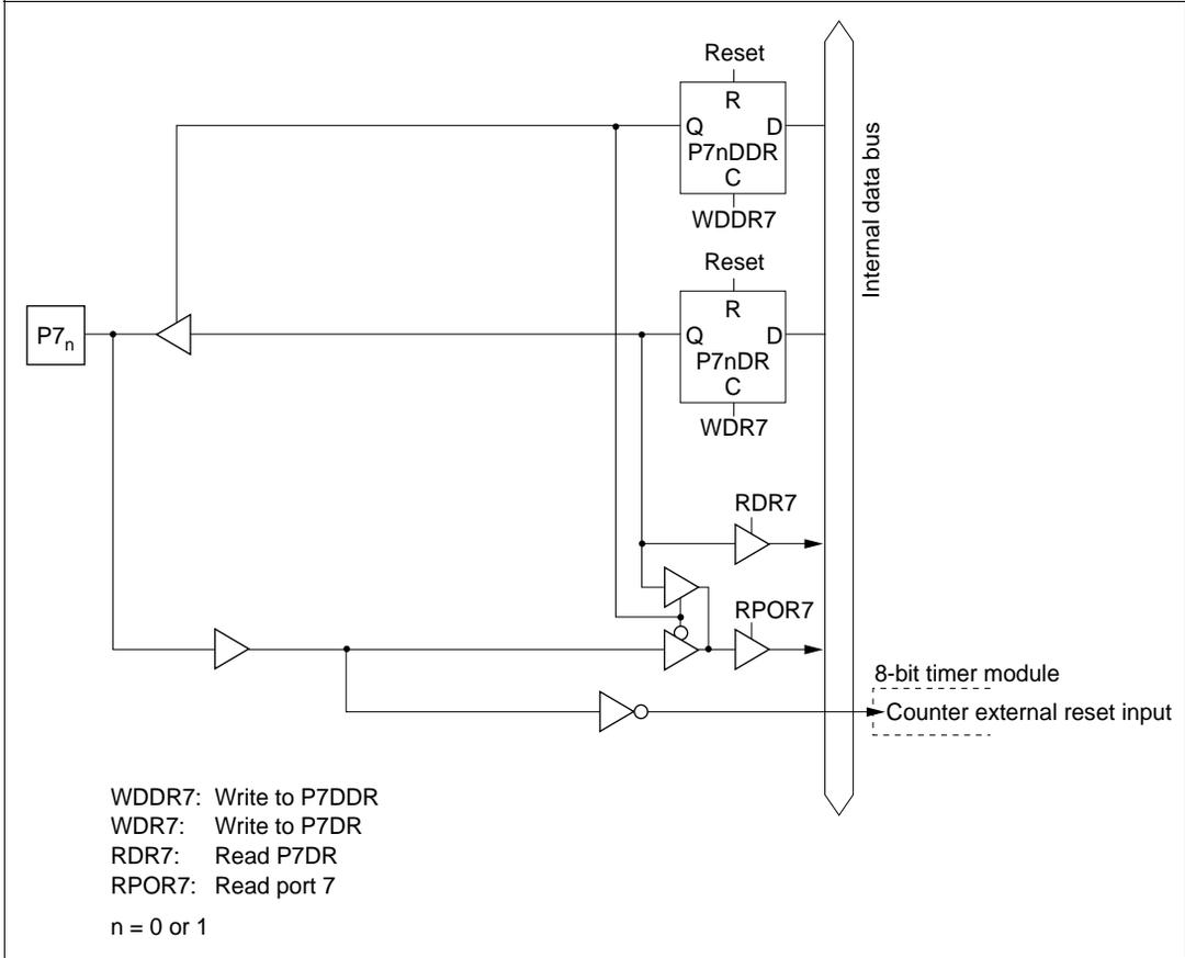
Figure 5.33 (a) Port 7 Block Diagram (Pins P7<sub>0</sub> and P7<sub>1</sub>)
