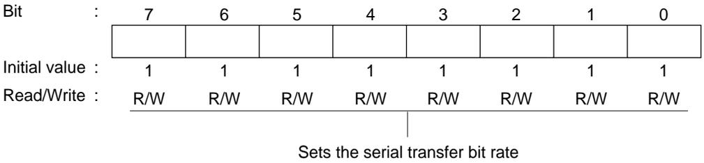
Note: For details, see section 11.2.8, Bit Rate Register (BRR), in the Hardware Manual.
