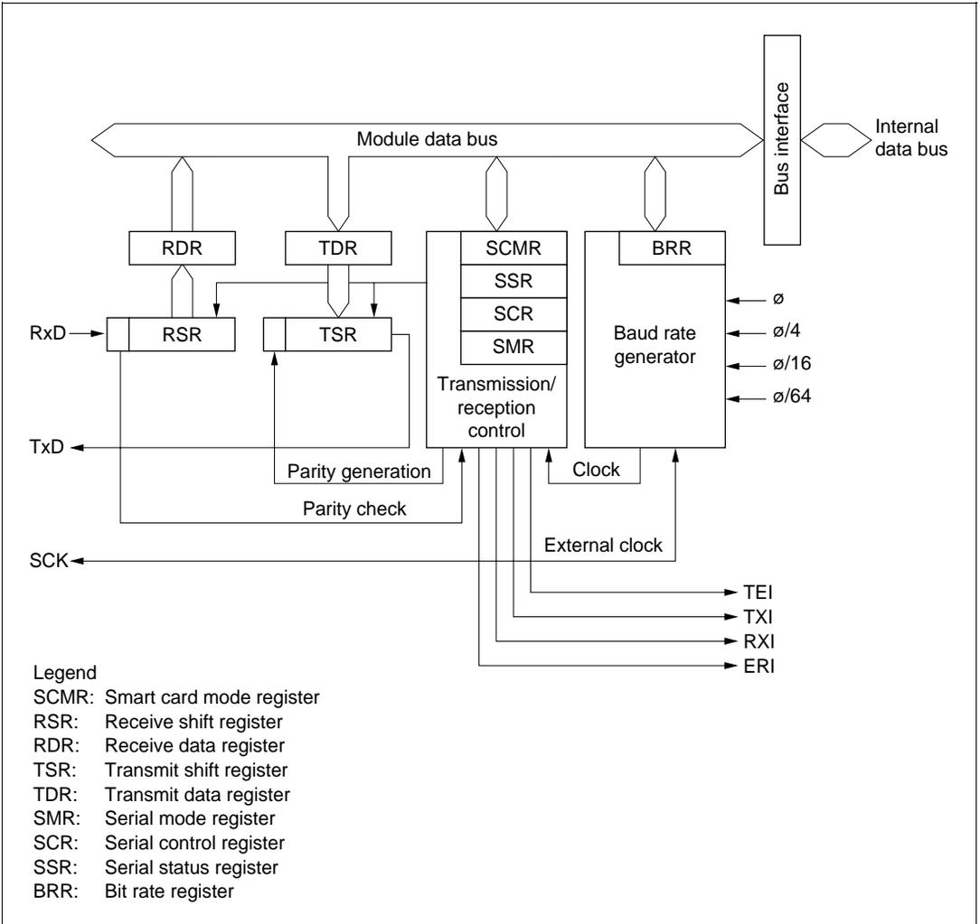
**Figure 6.8 Block Diagram of SCI**
