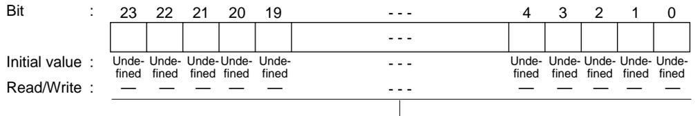
Specifies DTC transfer data source address
