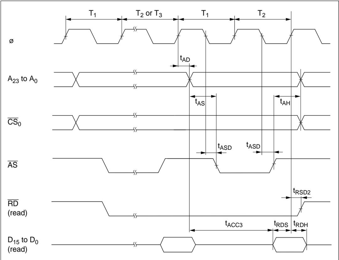
**Figure 7.12 Burst ROM Access Timing (2-State Access)**
