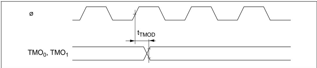
**Figure 7.24 8-Bit Timer Output Timing**
