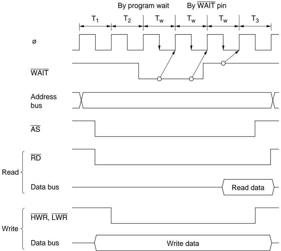
Note: Downward arrows indicates the timing of  $\overline{\text{WAIT}}$  pin sampling.
