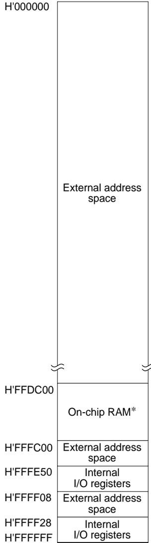
Note: \* External addresses can be accessed by clearing the RAME bit in SYSCR to 0.
