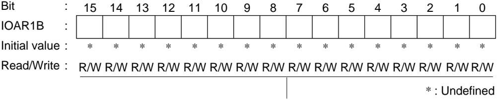
In short address mode: Specifies transfer source/transfer destination address
