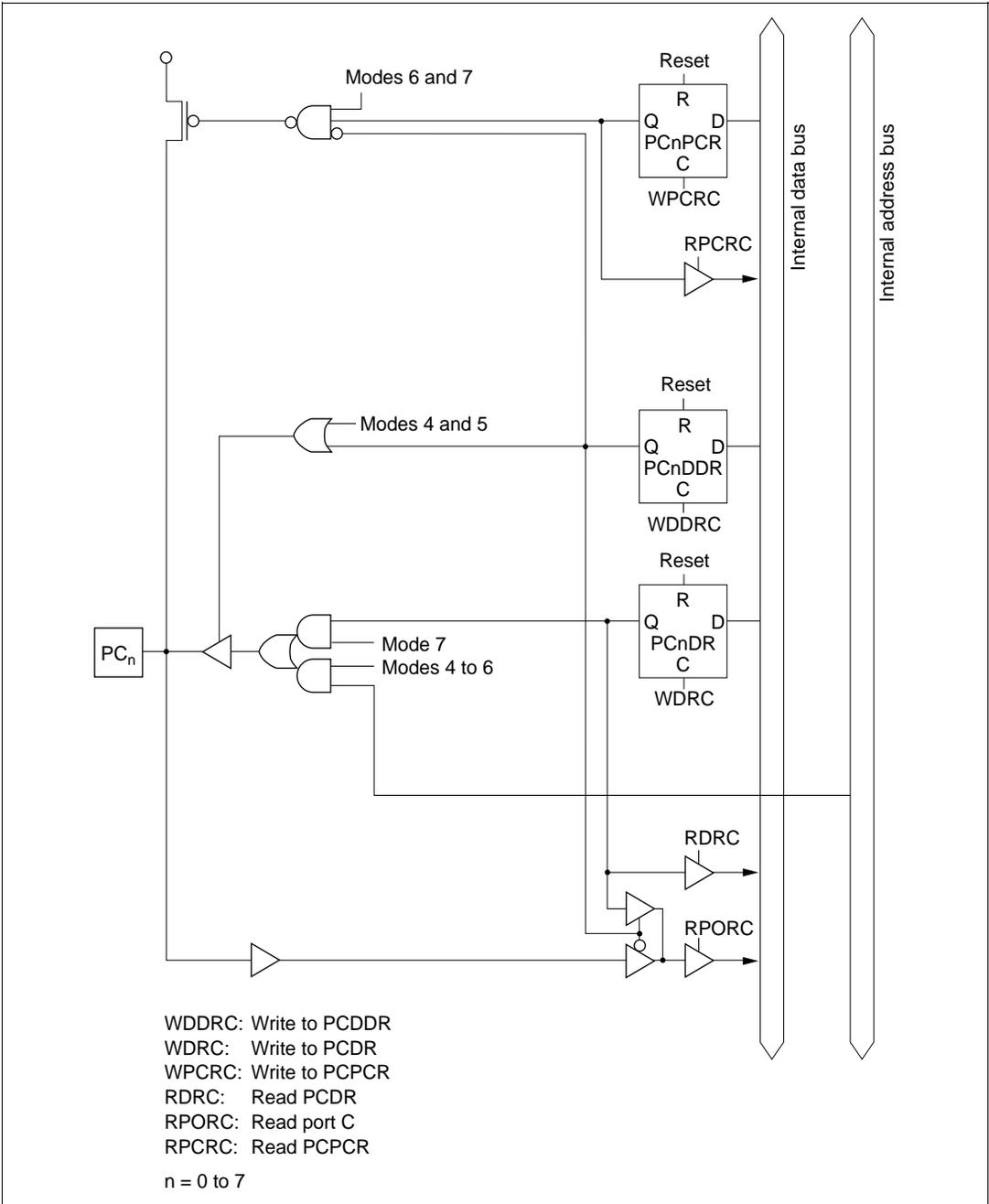
Figure 5.38 Port C Block Diagram (Pins PC<sub>n</sub>)
