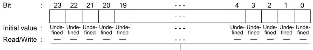
Specifies DTC transfer data destination address
