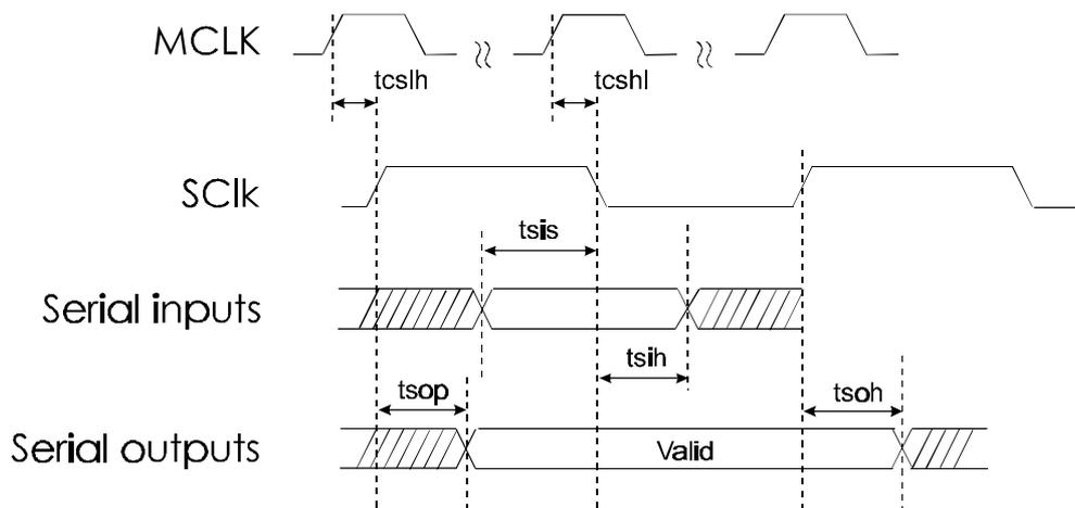
Figure 4 Serial Port Interfaces - Timing Parameters
