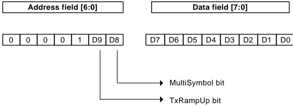
**Address and Data format for TxData (Modulator Bypass Mode) Write access**
