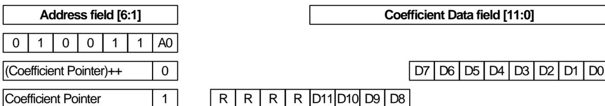
• Address and Data format for 79-tap Tx FIR Coefficient Ram IO access
