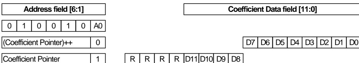
• Address and Data format for 49-tap Tx FIR Coefficient Ram IO access
