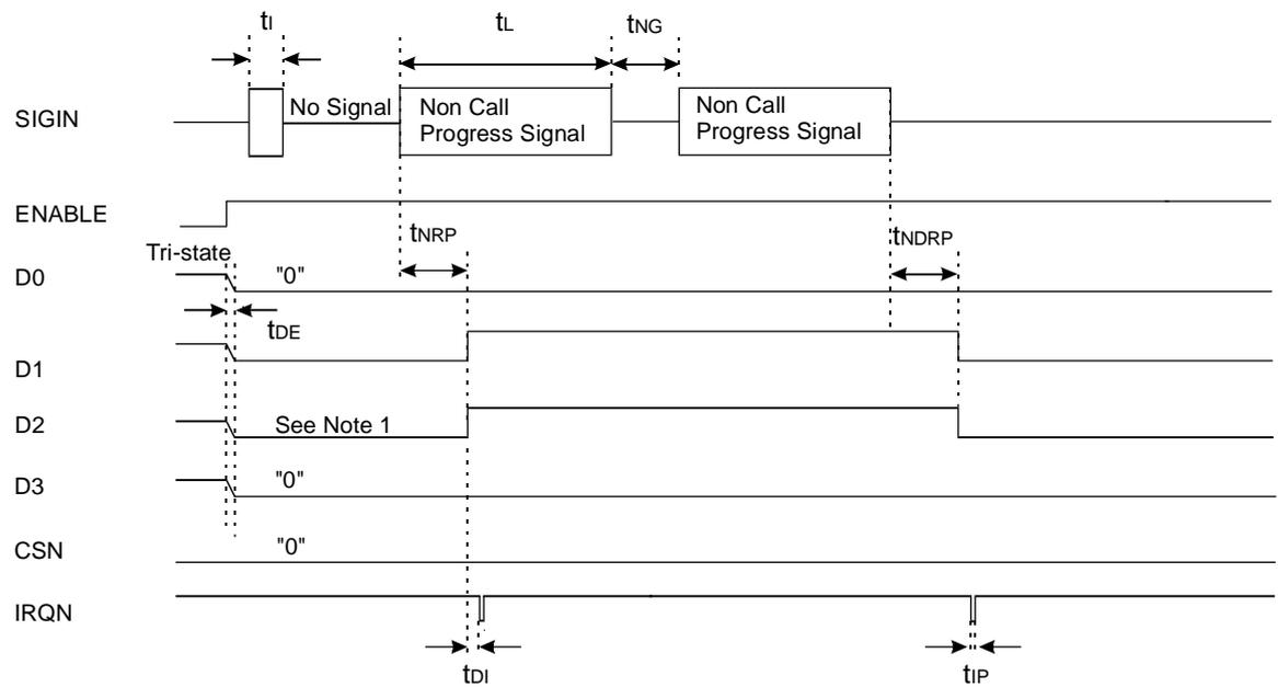
Figure 5 Timing Diagram: Non Call Progress Signal
