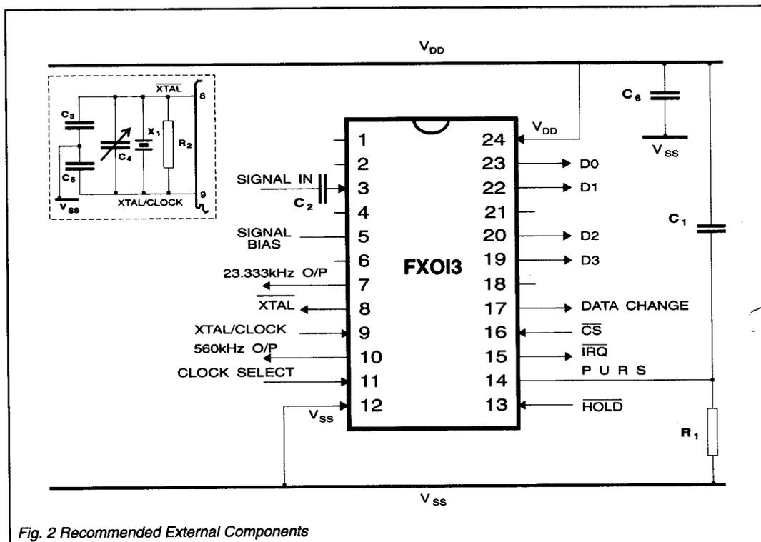
Fig. 2 Recommended External Components
