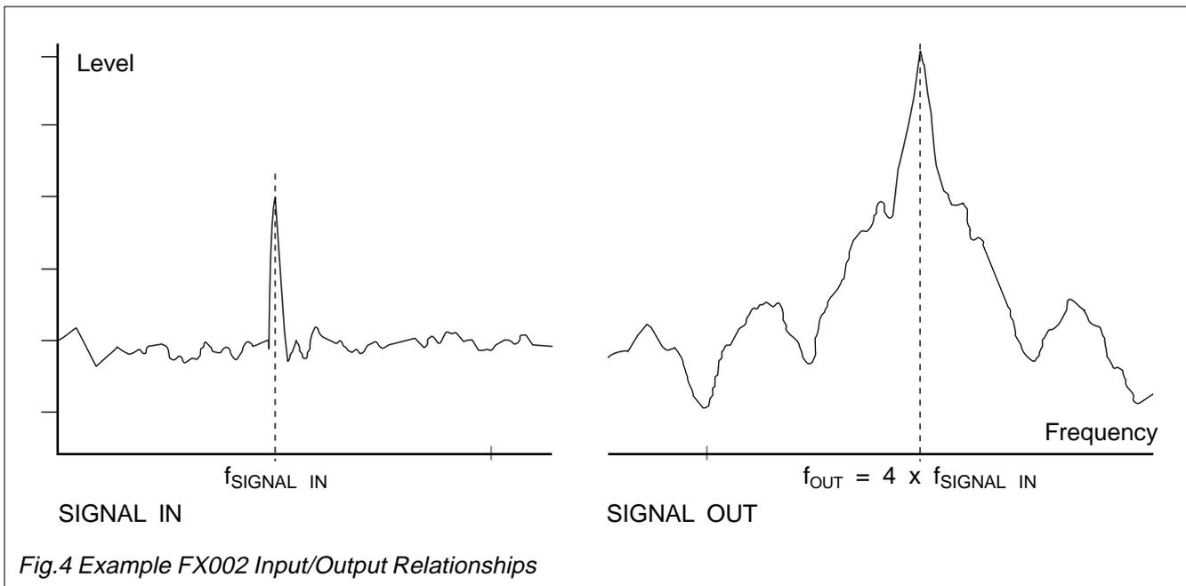
The diagrams in Figure 4 are example spectrums of the input and output signal conditions of the FX002. Note that the frequency of the output signal is four times (x4) that of the input signal.
