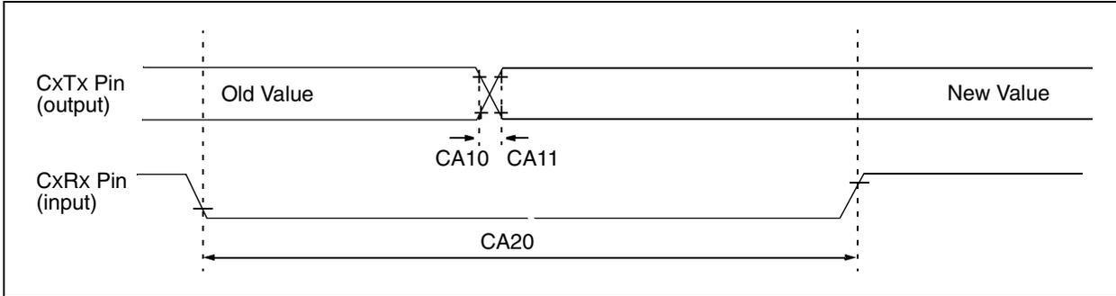
**TABLE 24-35: CAN MODULE I/O TIMING REQUIREMENTS**
