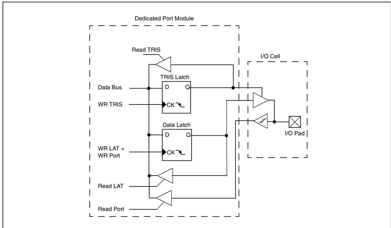
**FIGURE 8-2: BLOCK DIAGRAM OF A SHARED PORT STRUCTURE**
