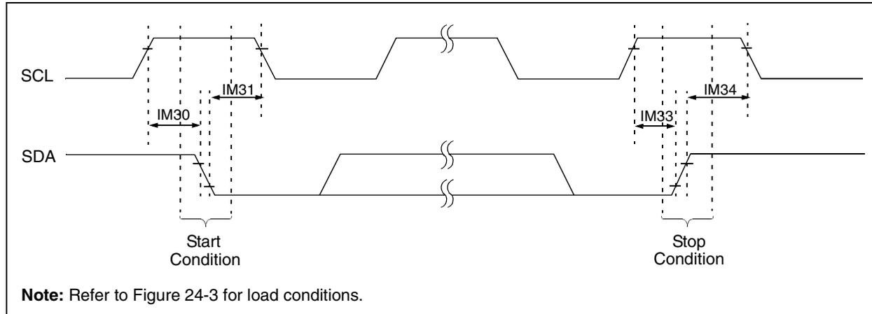
**FIGURE 24-22: I<sup>2</sup>C BUS DATA TIMING CHARACTERISTICS (MASTER MODE)**
