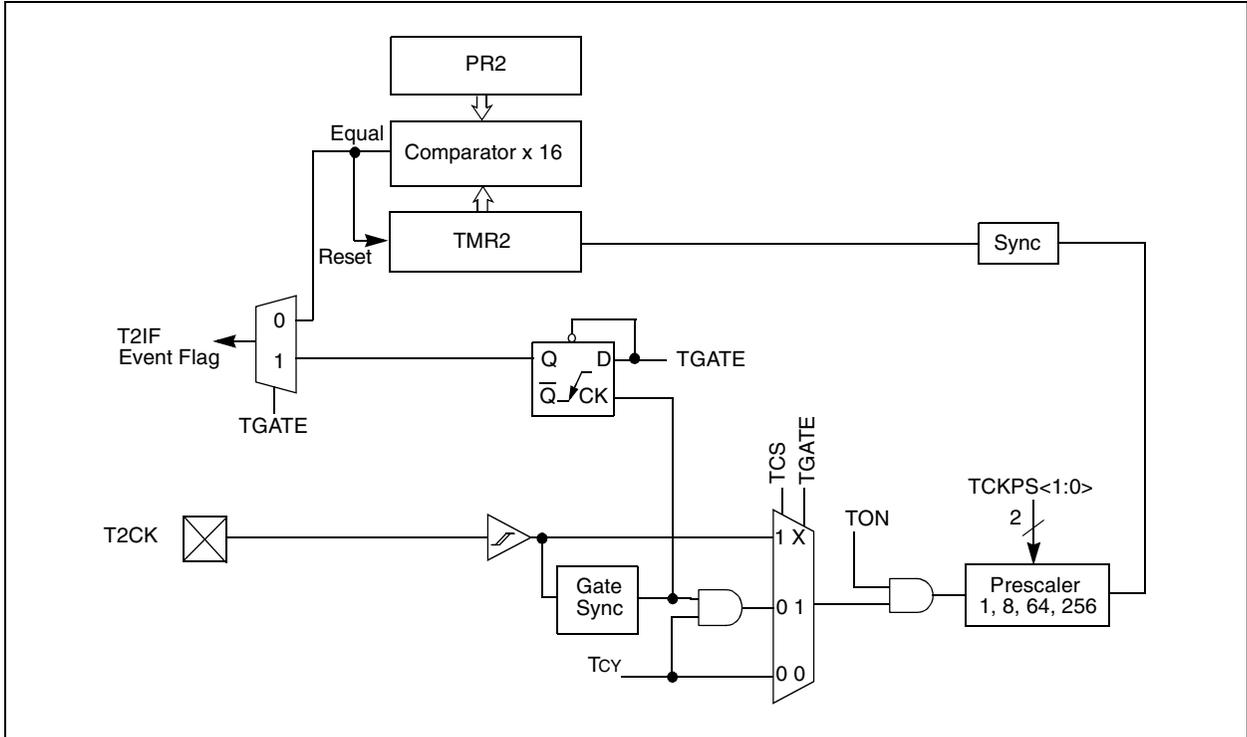
**FIGURE 10-3: 16-BIT TIMER3 BLOCK DIAGRAM (TYPE C TIMER)**
