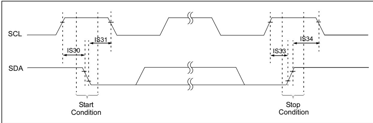
**FIGURE 22-23: I<sup>2</sup>C BUS DATA TIMING CHARACTERISTICS (SLAVE MODE)**
