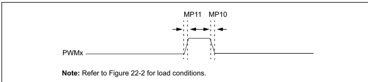
**TABLE 22-24: MOTOR CONTROL PWM MODULE TIMING REQUIREMENTS**
