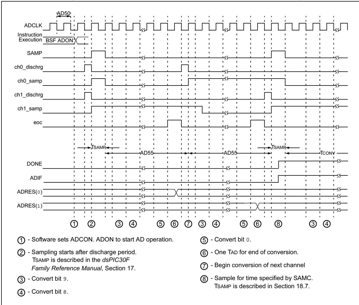
**TABLE 22-34: 10-BIT HIGH-SPEED A/D CONVERSION TIMING REQUIREMENTS**
