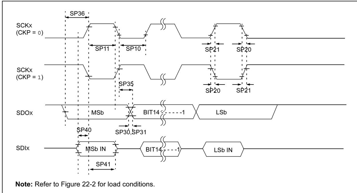
**TABLE 22-28: SPI MODULE MASTER MODE (CKE = 1) TIMING REQUIREMENTS**
