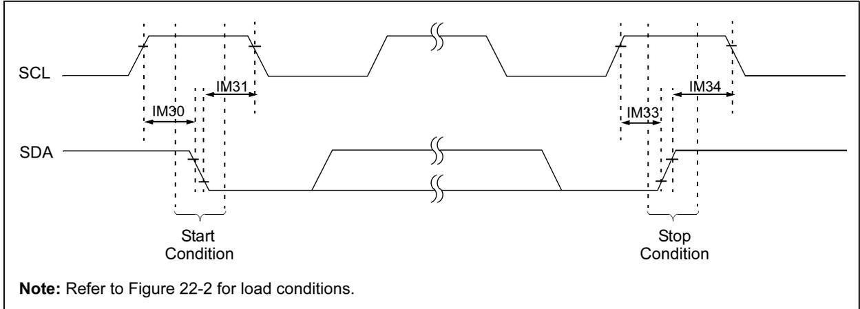
**FIGURE 22-21: I<sup>2</sup>C BUS DATA TIMING CHARACTERISTICS (MASTER MODE)**
