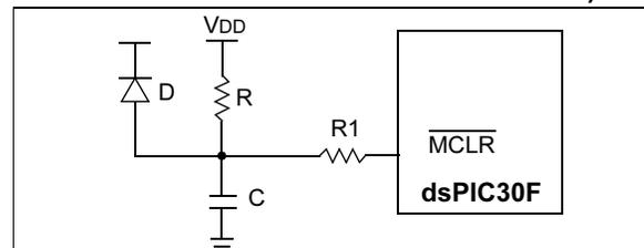
**Note 1:** External Power-on Reset circuit is required only if the VDD power-up slope is too slow. The diode D helps discharge the capacitor quickly when VDD powers down.
