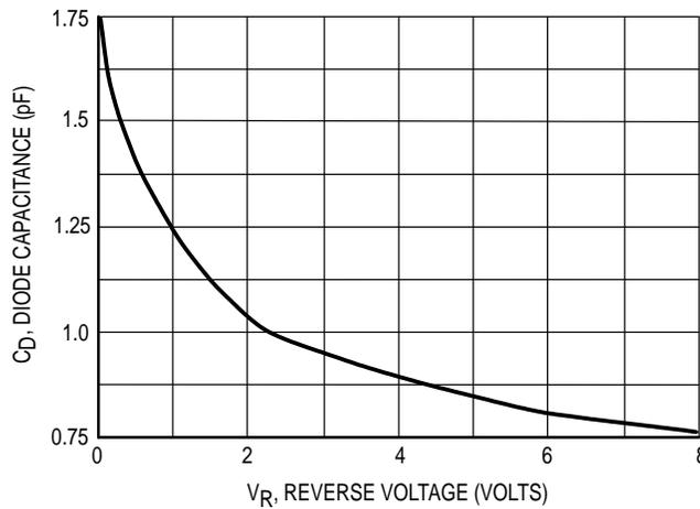
Figure 3. Diode Capacitance
