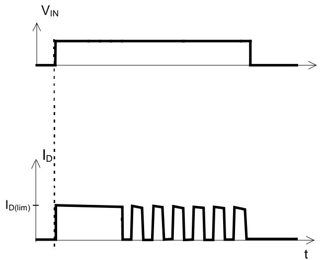
Shut down by overtemperature and restart by cooling. Current internally limited at  $I_{D(\text{lim})}$ .
